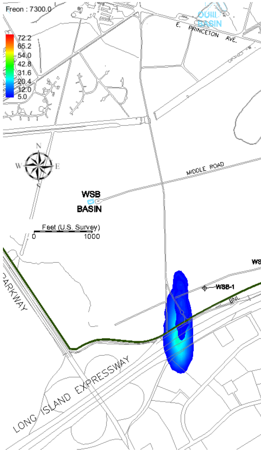
Figure 17 – Freon-12 Plume Under Natural Attenuation after 20 years (Year 2038)
