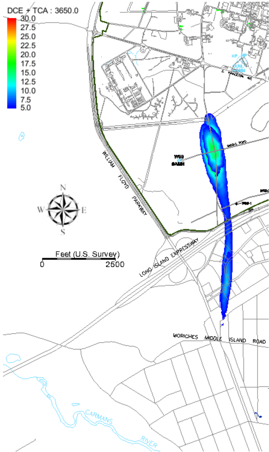
Figure 4 – DCE/TCA Plume Under Natural Attenuation after 10 years (Year 2028)
