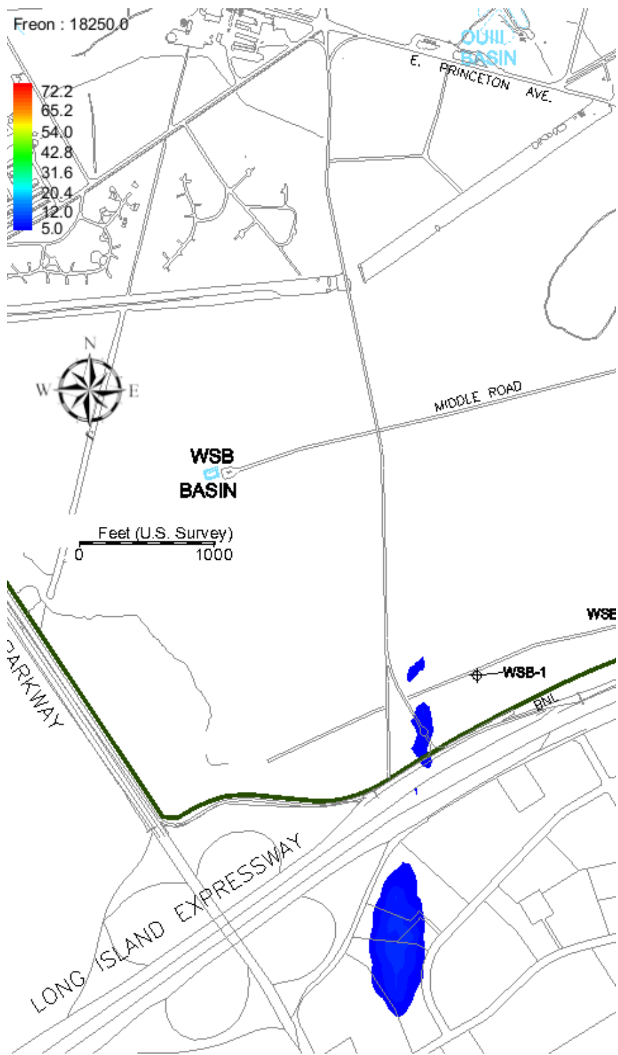
Figure 20 – Freon-12 Plume Under Natural Attenuation after 50 years (Year 2068)
