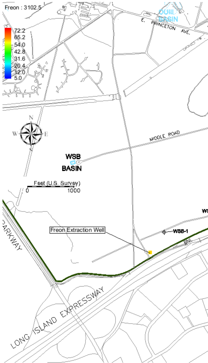
Figure 23 – Freon-12 Plume One New Extraction Well at 75 gpm – 8.5 years (Year 2026)
