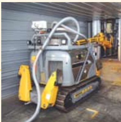
From left to right: Removal of the pile fan sump, remotely operated robot known as a BROKK manipulator, removal of the aboveground air ducts
