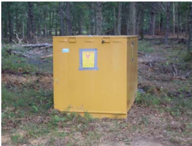
Photograph 4 – B-25 shipping container containing waste soil prior to shipment to Energy Solutions of Utah.
