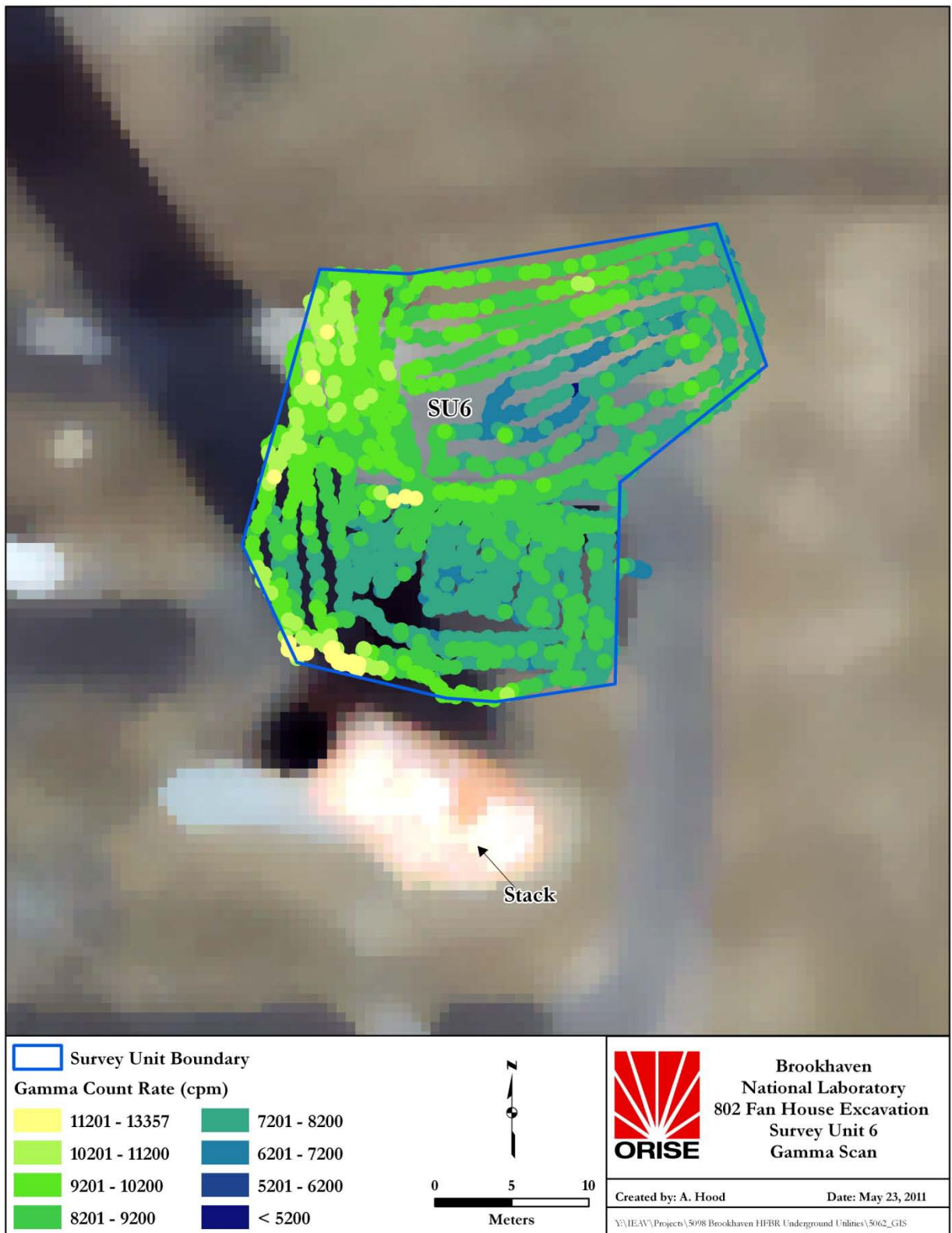
Figure A-6: Gamma Scans of the 802 Fan House Survey Area
