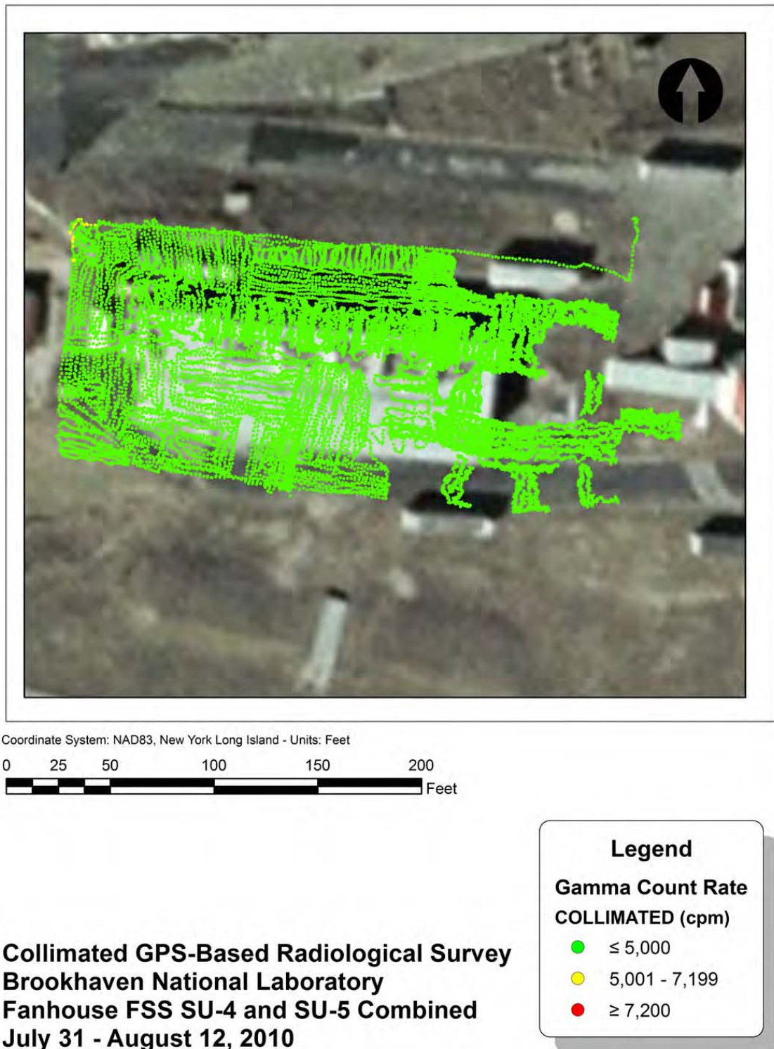
Figure 3-6– SU-4 and SU-5 Gamma Walkover Survey Results (Collimated Probe)
