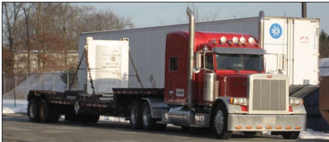
Figure 3-13. CNS 1-13G shipping cask with CRBs ready for the road.
