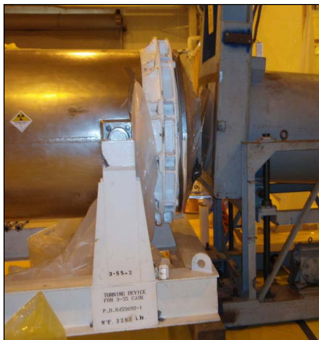
Figure 3-14. Transfer of BP H-9 to shipping cask CNS 3-55.
