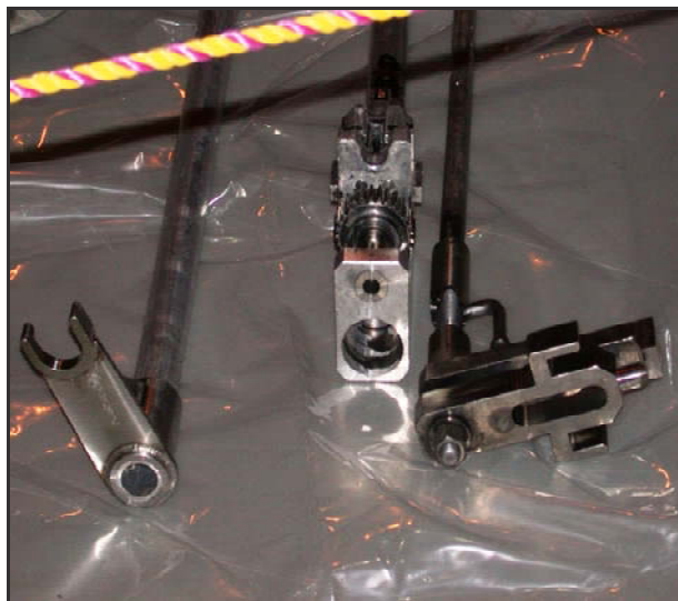
Figure 3-2. Close-up view of CRB tools (left to right): auxiliary blade guide bushing tool, main and auxiliary blade (un)coupling tool, main blade handling tool.
