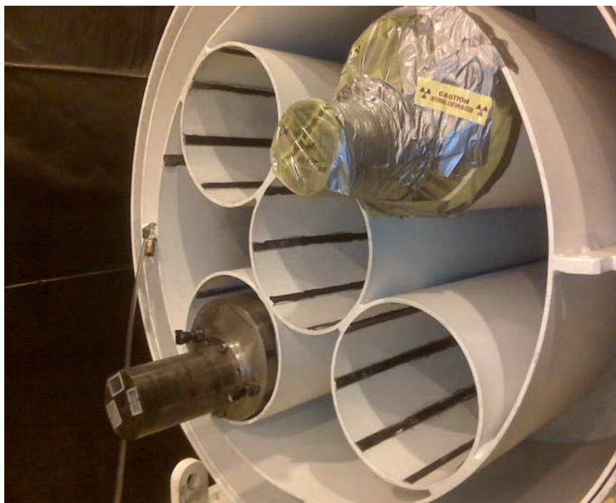
Figure 3-18. BP loading configuration of partially loaded 10-142 cask.
