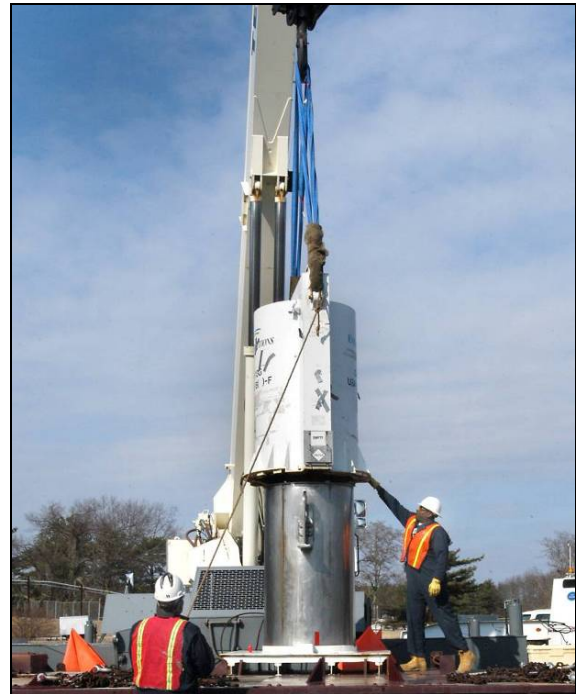
Figure 3-12. Shielded overpack being placed over CNS 1-13G cask.
