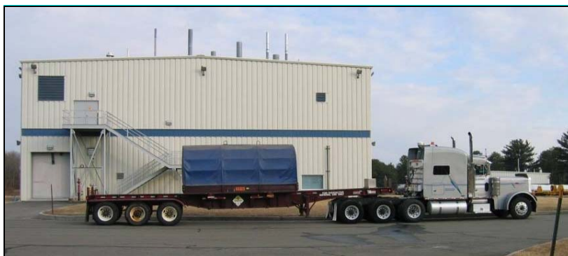
Figure 3-16. H-9 in CNS 3-55 cask ready for shipment.
