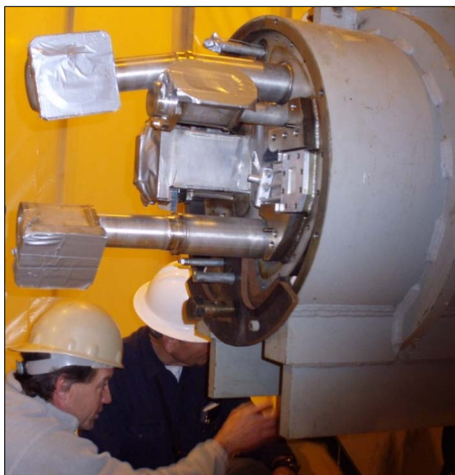
Figure 3-15. BP H-9 being loaded into shipping cask CNS 3-55.
