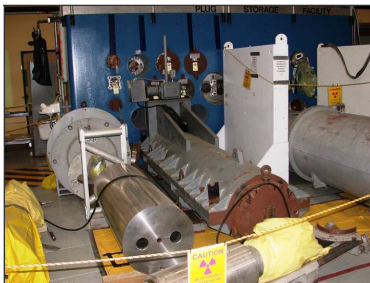
Figure 3-4 Beam plugs, transfer casks, and BP storage area at start of BP and collimator removal.
