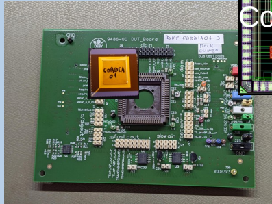
analog chain (preamplifier + S/H + CDS), Adaptive Gain operation
