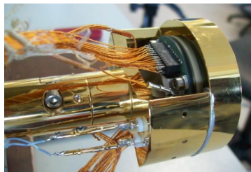
Front-end board with 19 CUBE preamplifiers
