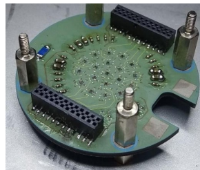
Front-end board with 19 CUBE preamplifiers
