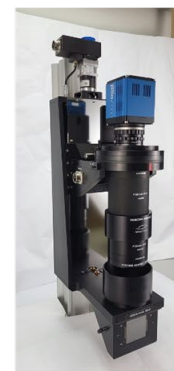
Macroscopes (2x..0.5x) Custom made high NA high resolution lenses
