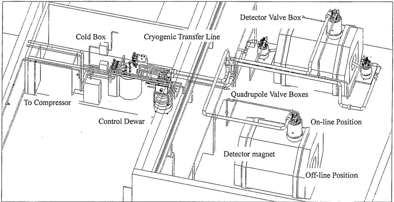
Figure 2 The first colliding hall and its cryogenic system
