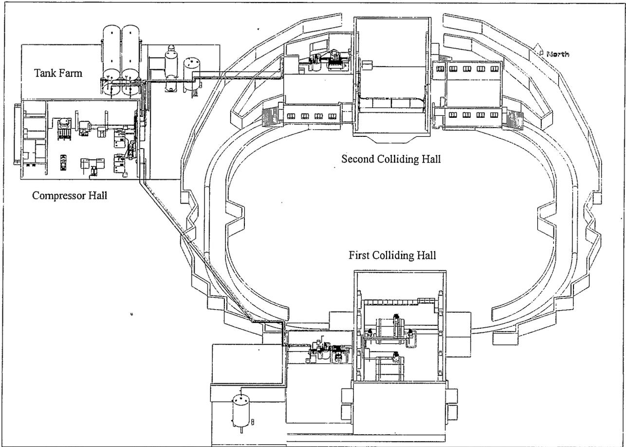
Figure 1 BEPCII ring and its cryogenic facilities
