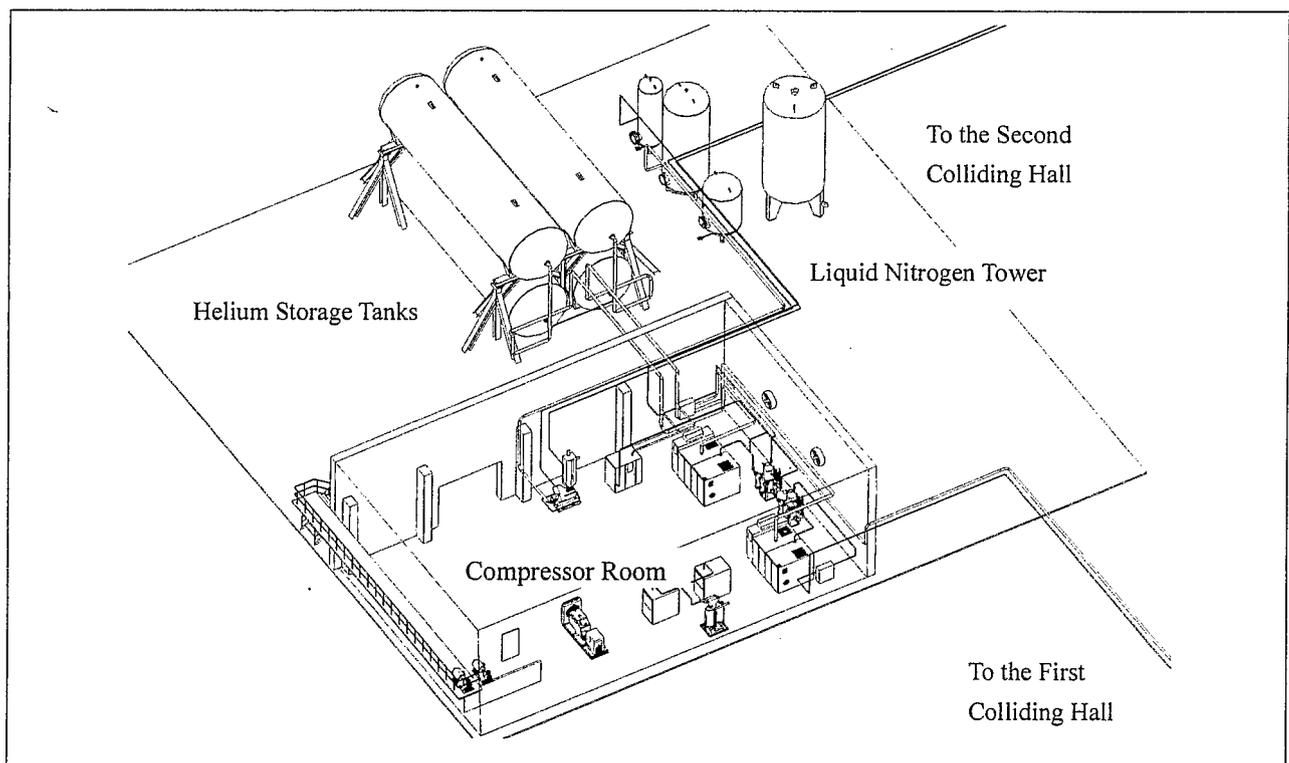
Figure 4 Compressor room and gas tank farm
