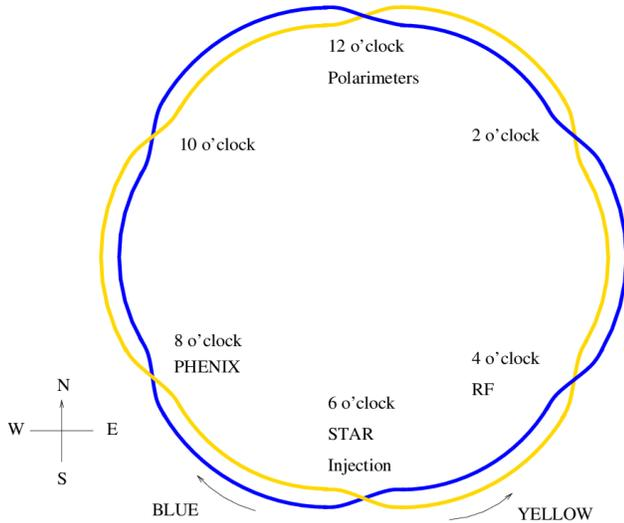
Figure 1: Schematic view of RHIC with its two intersecting storage rings.
