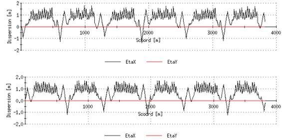
Figure 3: Dispersion functions in the “Blue” (top) and “Yellow” RHIC rings right before the transition jump.
