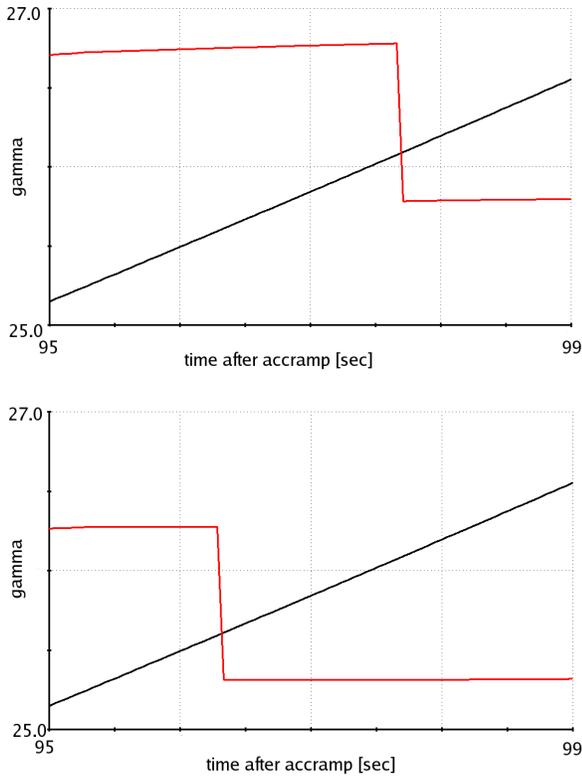
Figure 4: Beam energy  $\gamma$  (black) and transition energy  $\gamma_t$  (red) vs. time since “accramp”, in the “Blue” (top) and “Yellow” ring (bottom).
