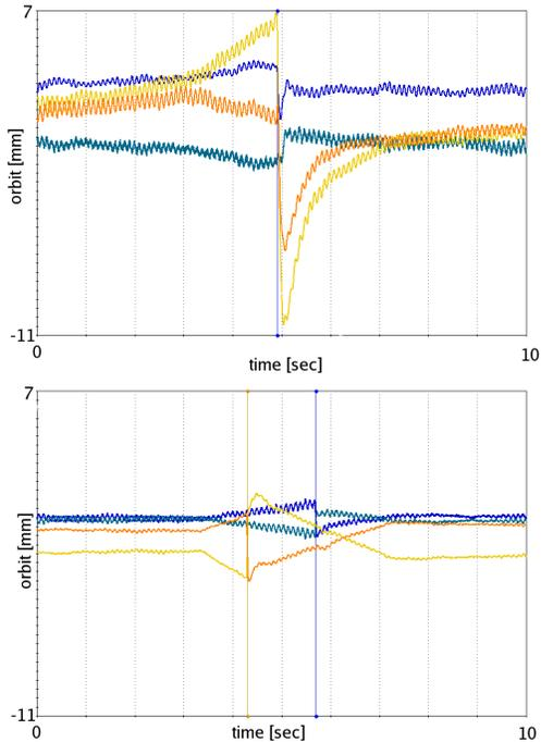
Figure 5: Radial loop BPM signals around transition, in FY07 (top) and FY10 (bottom).
