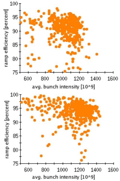
Figure 6: Ramp efficiencies in the “Yellow” ring, for equal transition times in FY07 (top), and split transition times in FY10 (bottom).
