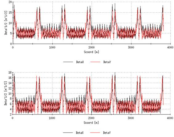
Figure 2:  $\beta$ -functions in the “Blue” (top) and “Yellow” RHIC rings right before the transition jump.
