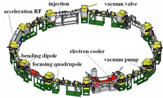
Table 1: Small storage ring (CRYRING at the Manne Siegbahn Laboratory) with main components labeled.
