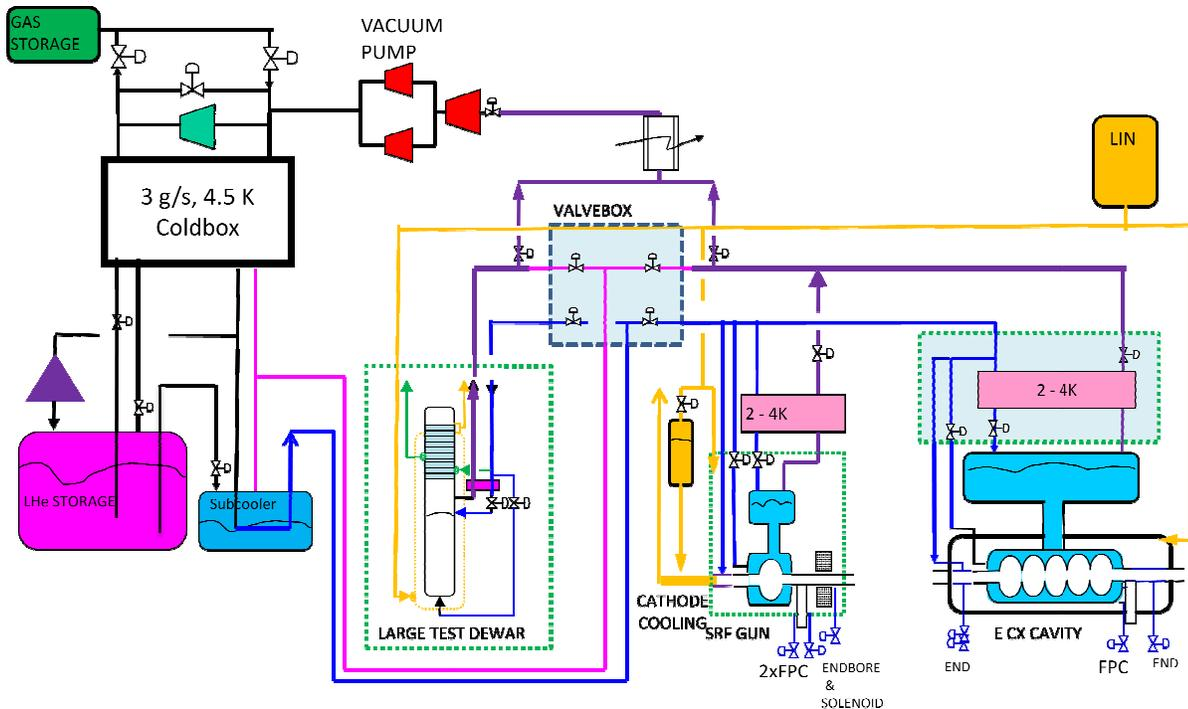
Figure 1: Process Flow Diagram Cryogenic System for Energy Recovery Linac and Vertical Test facility
