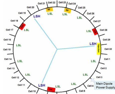
Figure 1 The modified storage ring layout with 3-fold symmetry. LSH represents long straight with high horizontal beta function; LSL represents long straight with low horizontal beta function.
