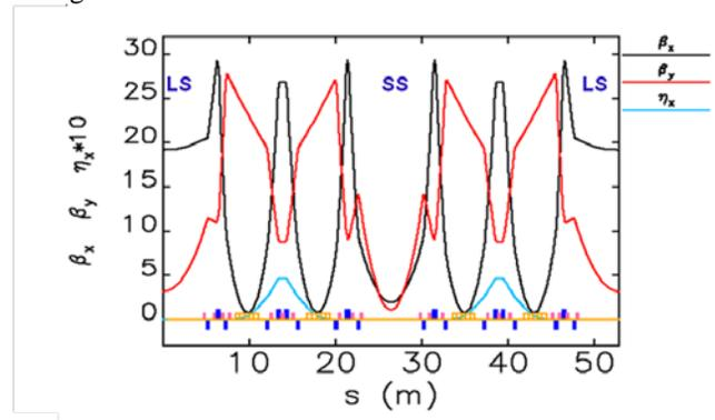
Figure 2 The baseline lattice functions for two DBA cells (LS: long straight; SS: short straight).
