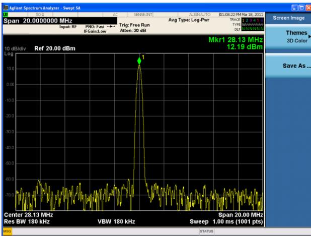
Figure 3: Broad band spectrum of DDS output at 28 MHz BlockRAM. Meeting timing in the FPGA at 400 MHz was extremely challenging.
