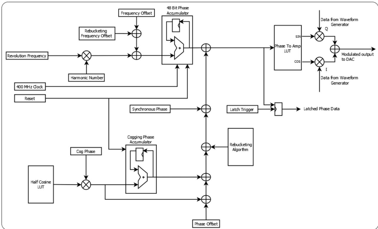
Figure 1: Simplified block diagram of DDS implementation.
