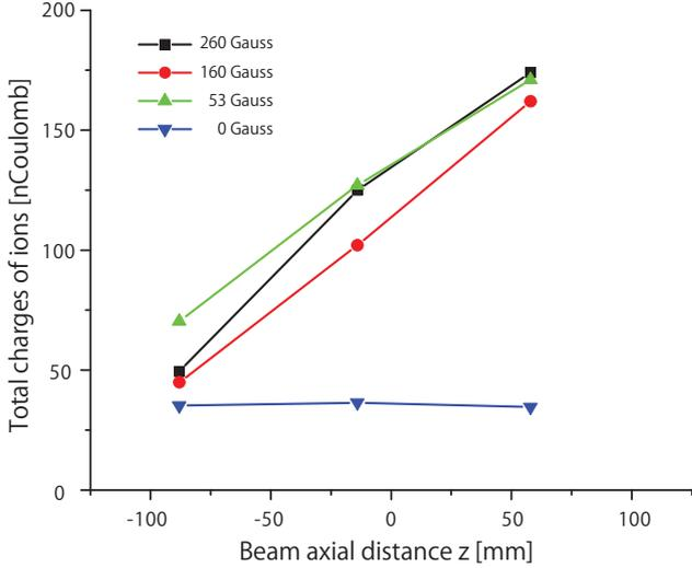
Figure 7: Total charges of ions for magnetic field strength vs Axial position. The total charges with magnetic field (black, red, and green lines) decay with distance from the end of solenoid.
