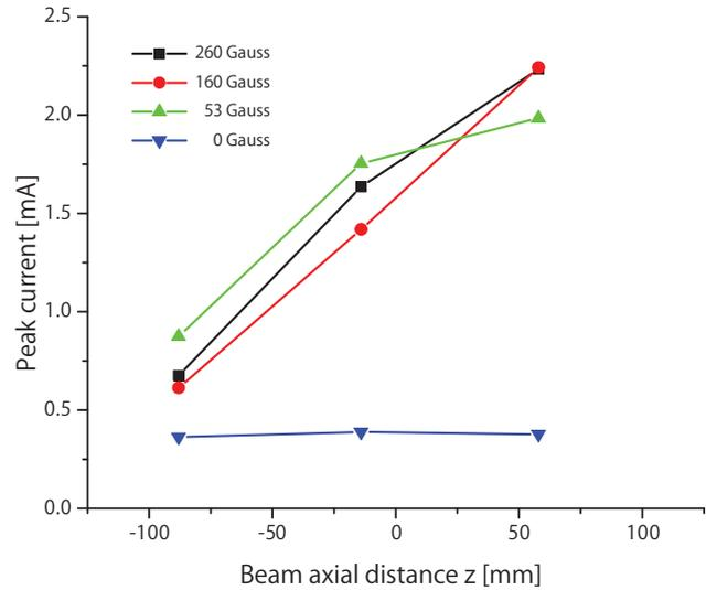
Figure 5: Peak current for magnetic field strength vs beam axial distance. No magnetic field represents blue line and that is constant for z position.
