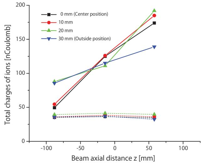
Figure 4: These lines show total ion charges for radial position with beam axial distance. Solid lines are for maximum magnetic field of 260 Gauss and dash lines are for no magnetic field. Each color represent a radial position from the center of beam.
