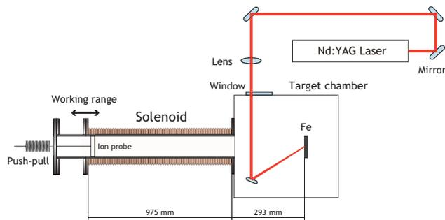
Figure 1: LIS experimental setup sketch. The push-pull allows the ion probe to be moved along the beam axis.
