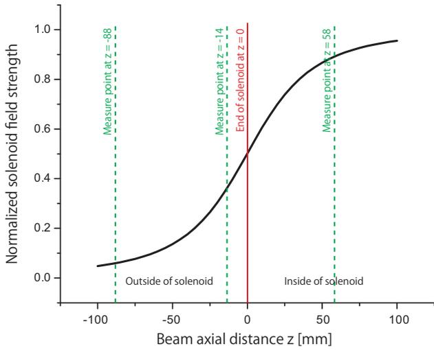
Figure 3: Normalized magnetic distribution around the end of solenoid (red line) and three scanned positions of the beam axis (green dash lines).
