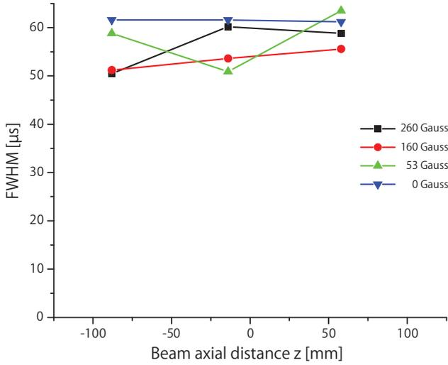
Figure 6: FWHM of beam pulse length for magnetic field strength vs Axial position. The results show no dependence on field strength.
