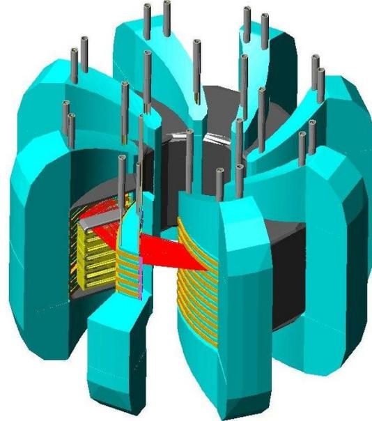
Figure 2. Isotropic cutaway view of a flux-coupled 7-stack of isochronous cyclotrons. The proton orbits in the top IC are shown in red.
