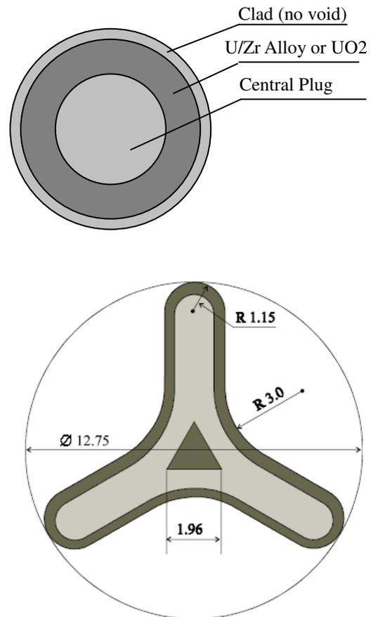
**Figure 3.** Seed Fuel Rod Geometry for PWR and VVER
