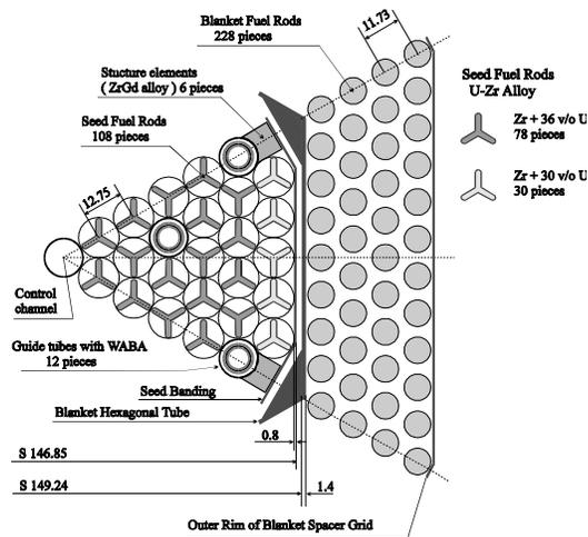
**Figure 2.** SBU Geometry for VVER
