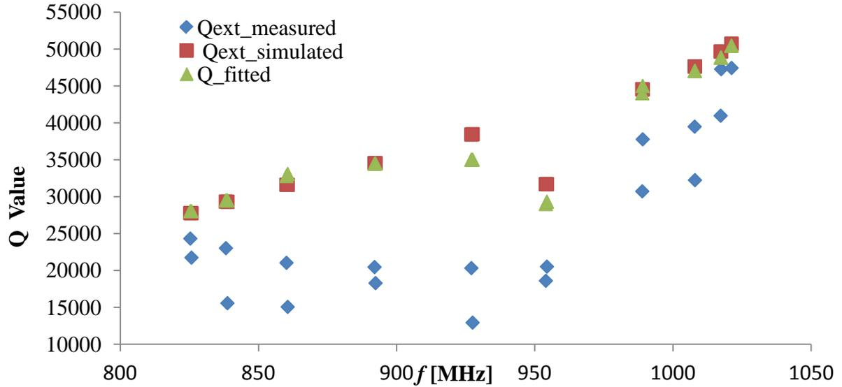
FIG.11: Comparison results from measurement, simulation and fitting results of BNL3 cavity
