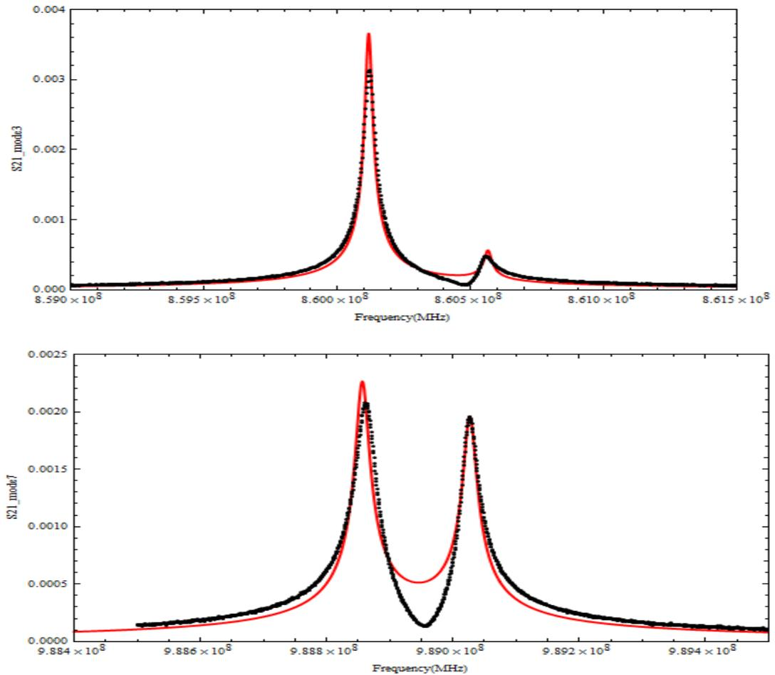
FIG. 12: S<sub>21</sub> fitting results. Black dot: measured data; Red curve: fitting curve
