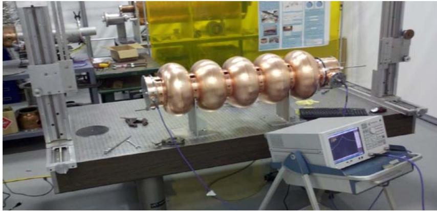
FIG. 1: Setup of the measurement with closed beam pipe
