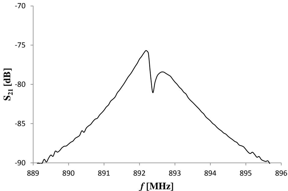
FIG. 6: Typical  $S_{21}$  curve of the splitting modes
