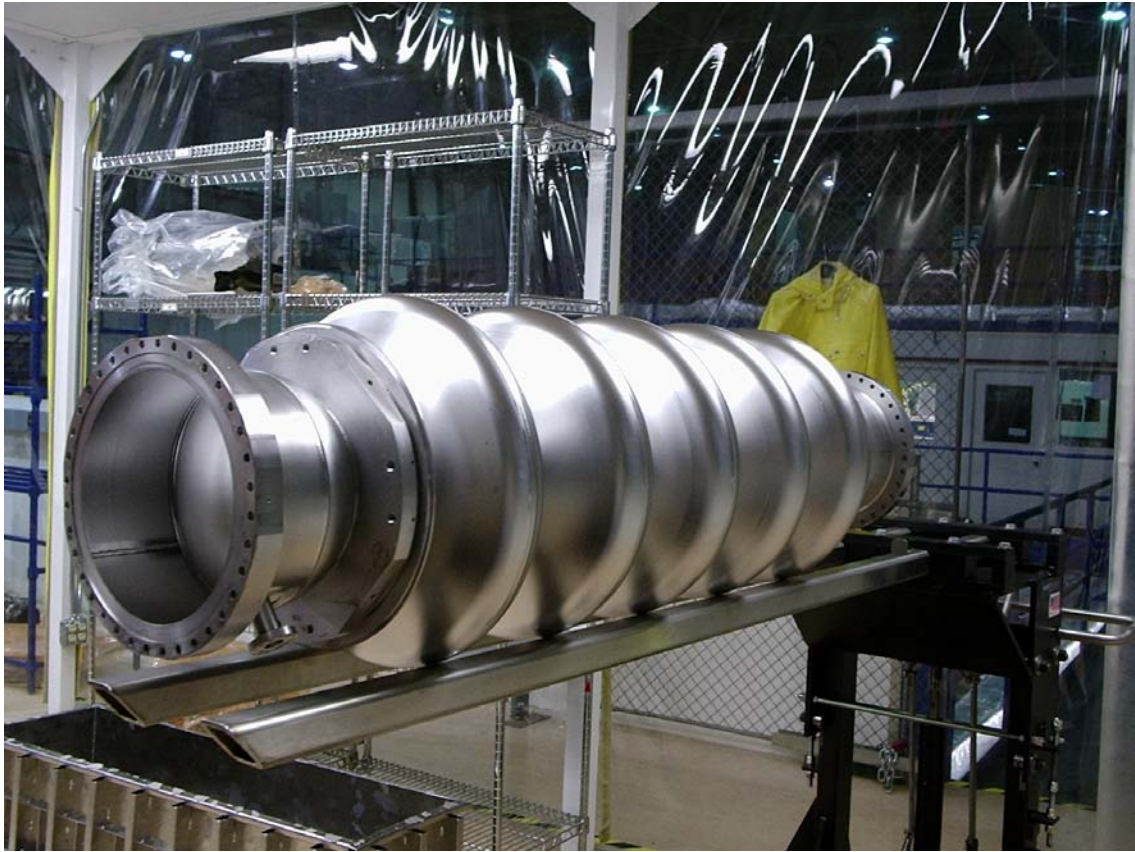
Figure 7. The ERL 5-cell accelerating cavity.
