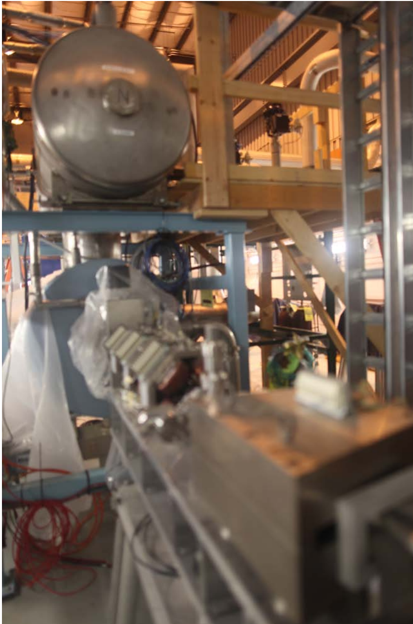
Figure 8. The linac cryomodule of the ERL and part of the 20 MeV beam line.
