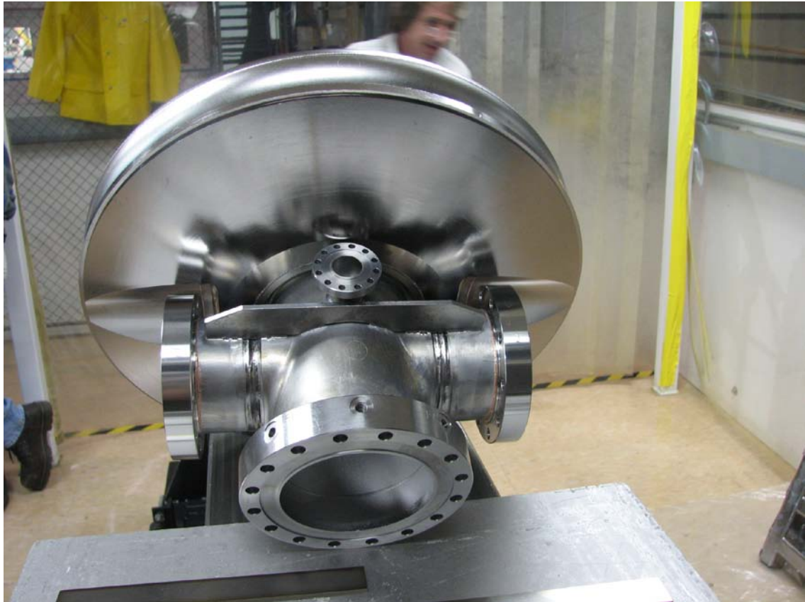
Figure 5. SRF photocathode electron gun, 2 MeV 300 mA at 704 MHz. The beam port faces front, the twin fundamental power couplers to the right and left, the pick-up probe facing upwards.
