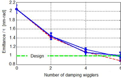
Figure 6: Measurement of horizontal emittance vs. number of damping wigglers with a pin-hole X-ray monitor (blue: measurements, red: calculation)
