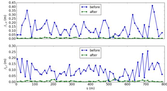
Figure 4: Local and global coupling correction: the mode-II  $\beta_{xII}$  and mode-I  $\beta_{yI}$  which represent the off diagonal blocks of the 4x4 revolution matrices at each element of the accelerator before and after correction.
