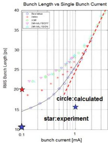
Figure 9: Measured and expected bunch lengthening in NSLS-II
