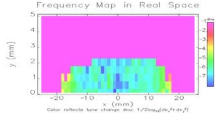
Figure 7: Frequency map of NSLS-II Dynamic Aperture (DA) in the x-y plane at injection point
