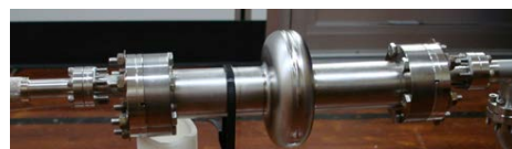
Figure 8: Top: 3D model of the 3.9 GHz 9-cell crab cavity for ILC. Bottom: Single-cell prototype.
