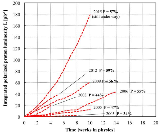
Figure 1: Integrated luminosity and polarization for all RHIC 100 GeV polarized proton runs.
