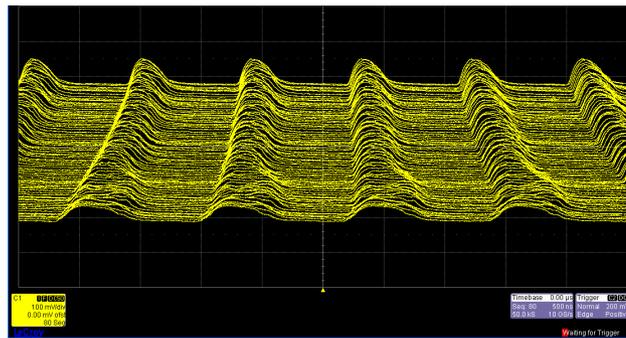
Figure 3: A mountain range of the Booster wall current monitor signal during early acceleration after capture using double-harmonic cavities to produce a longer, flat bunch distribution.
