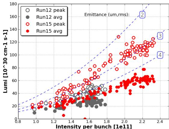
Figure 2: Peak and average luminosity for all stores as a function of bunch intensity. Peak luminosity in Run 12 saturated at  $50 \times 10^{30} \text{ cm}^{-1} \text{ s}^{-1}$  due to beam-beam induced emittance blowup. Electron lens compensation and improved off-momentum DA allowed higher luminosity in Run 15. The blue dashed lines are curves of constant emittance.
