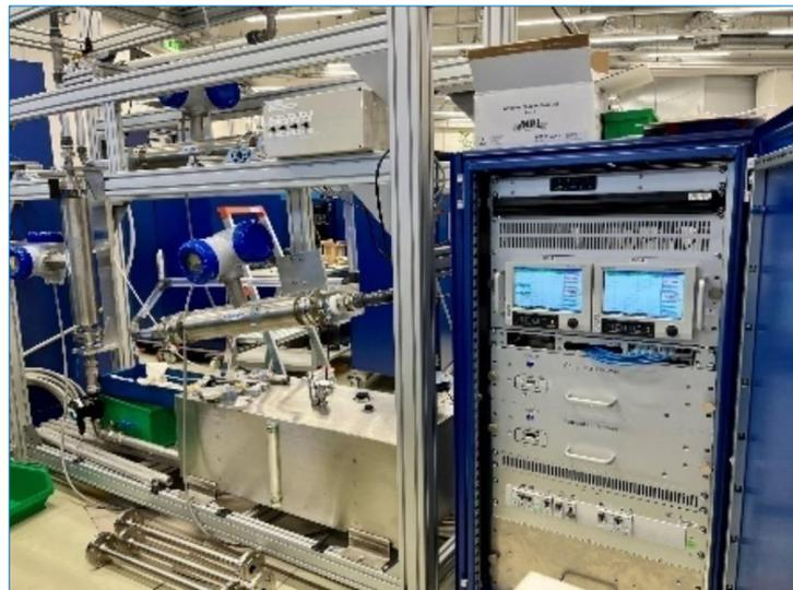
*Figure 75: Coriolis flow meter-based system undergoing a functional and technical performance evaluation at the UMS laboratory.*
