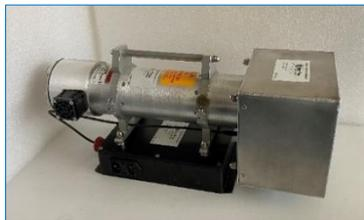
Figure 41: nGen-350 DD neutron generator for use as a neutron interrogation source with FNCL.
