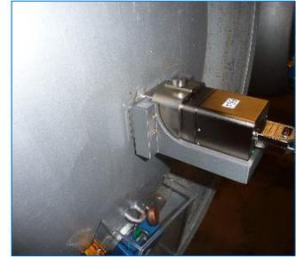
Figure 40: The MCCM attached to a cylinder is to be the “workhorse” of NDA tools for the foreseeable future.
