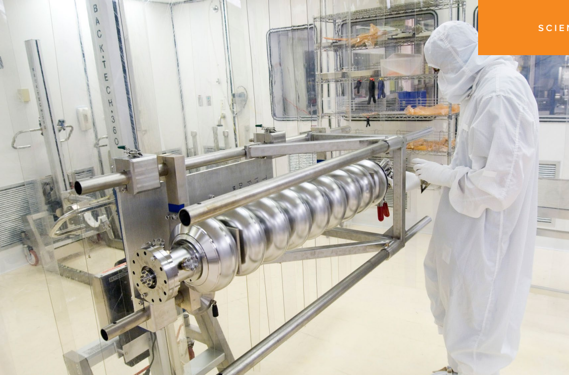
Technician in ultra-clean environment at Jefferson Lab preparing a superconducting radiofrequency cavity. (Credit: Thomas Jefferson National Accelerator Facility)
