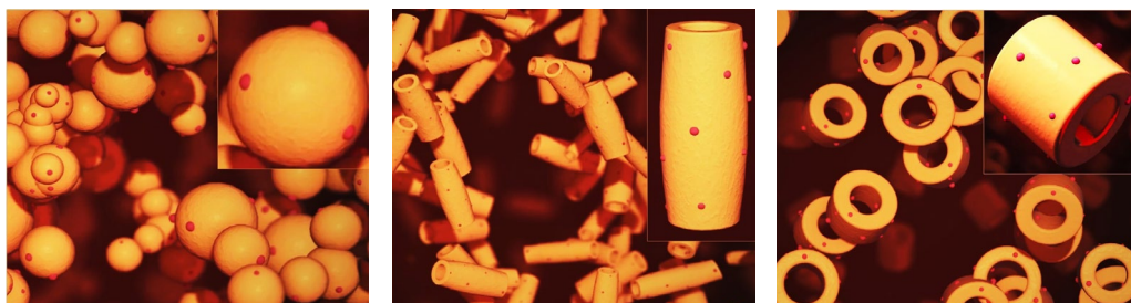
Shape-selective hybrid nano-antenna materials, including spheres (left), elongated tubes (middle), and equiaxed rings (orange) decorated with nanomaterials (red) (right). The nano-antennas are composed of combinations of plasmonic, magnetic, and/or hydride components. (Credit: Savannah River National Laboratory)
