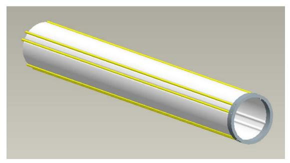
**Figure A3.3: Inner Heat Shield Assembly.** *Helium lines that are welded in place and the end manifold are shown.*
