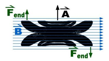
Figure 5.4: Force Diagram for a Horizontally Bending Dipole Coil Embedded in a Uniform Longitudinal Magnetic Field.
