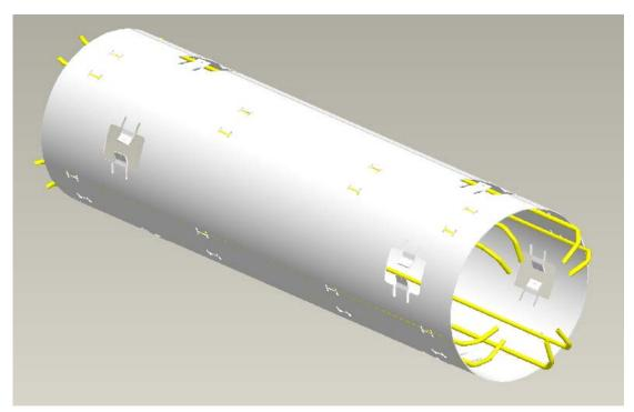
Figure A3.2: Outer Heat Shield Assembly. Helium lines that are welded in place and tabs for mechanical heat stationing of magnet supports are shown.
