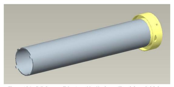
**Figure A3.1: Coil Support Tube Assembly.** Notches at IP end for radial helium passage between inner and outer flow annuluses, and flange pre-welded onto non-IP end are shown.
