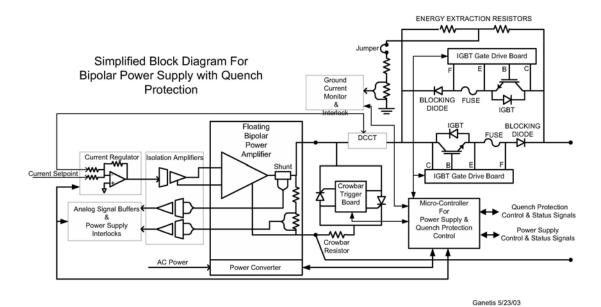
Figure A2.2: Bipolar Power Supply with Quench Protection.
