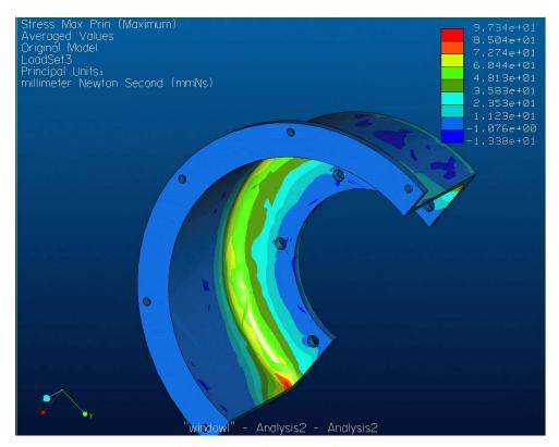
Figure 9.2: Axial Stress Outward.
