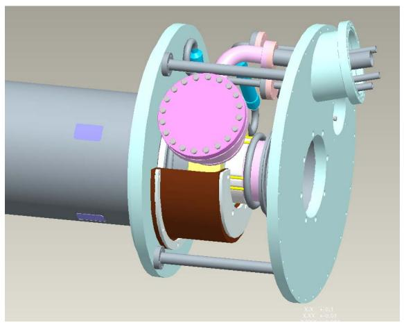
Figure 9.1: Axial Support Detail. Axial support (shown in brown) transmits longitudinal force from cold mass to endcan structure.
