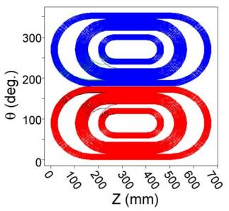
Figure 2.3: Sample Double Layer Dipole Coil Winding Pattern.
