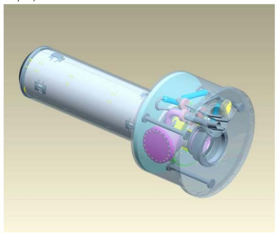
Figure 1.2: BEPC-II Superconducting IR Magnet 3-D Mechanical Model, non-IP End Isometric. The outer shells are shown translucent for clarity.
