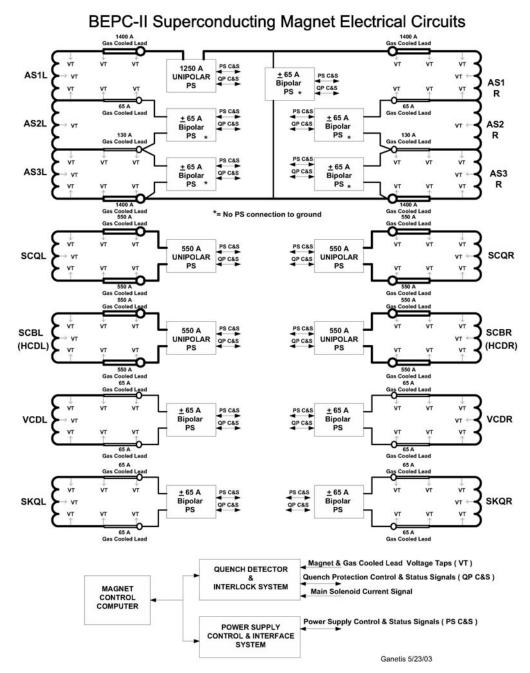
Figure A2.1: BEPC-II Superconducting Magnet Electrical Circuit.
