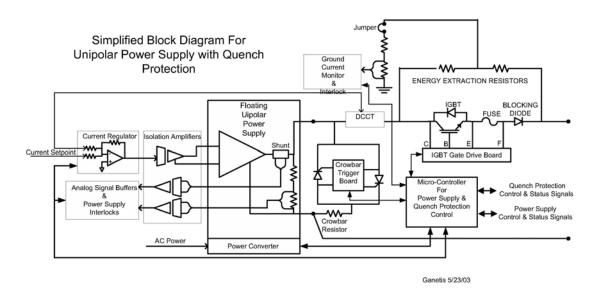
Figure A2.3: Unipolar Power Supply with Quench Protection.
