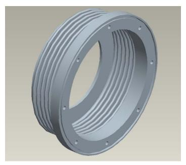
**Figure A3.5: Bellows Assembly.** The bellows assembly was recently increased in size to provide requested clearance volume of O190mm x 50mm at non-IP end.
