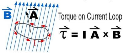
Figure 5.3: Convention for Calculating Torque for a Current Loop Embedded in a Uniform Magnetic Field.
