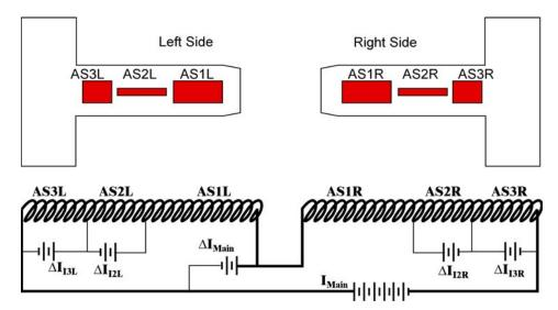
**Figure 4.2: Anti-Solenoid Power Schematic.** Main current of about 1120 A flows in series through all of the anti-solenoid coils. A small left-right asymmetry and small adjustments to the local compensation may be undertaken if additional trim current power supplies are provided but at the cost of additional current leads. Note that since the left and right cryostats are not directly connected independent current leads are needed on the IR right and left sides.
