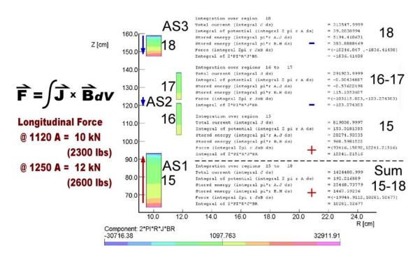
Figure 5.2: Anti-Solenoid Longitudinal Force Calculation.
