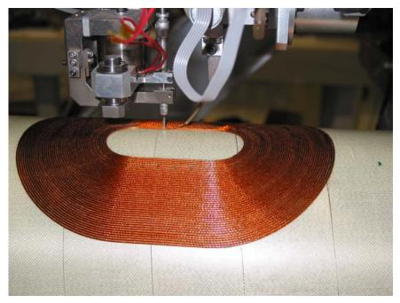
Figure 2.4: BEPC-II Test Coil Winding In Progress.
