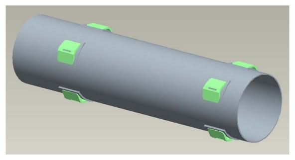
**Figure A3.4: Helium Containment Tube Weldment.** *G-10 magnet supports that are held in place by welded stainless steel retainers are shown.*
