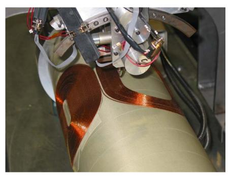
Figure 2.5: BEPC-II Test Coil Winding In Progress..
