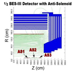
Figure 3.2: Three anti-solenoid subcoils, AS1-3 inside BES-III experimental detector. The anti-solenoid locally compensates BES-III detector field for the circulating beams. The anti-solenoid scheme is mirror symmetric about the vertical plane Z=0 and rotationally symmetric about the Z-axis.
