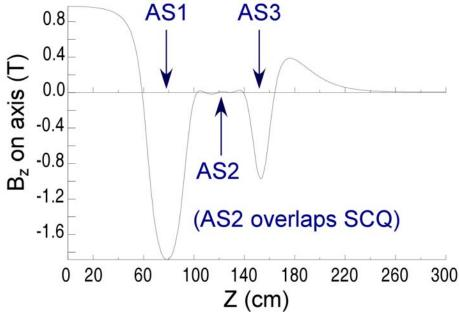
Figure 4.1: On Axis Local Compensation of BES-III Detector Solenoid Via a Three Part Anti-Solenoid.
