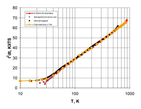
Figure A1.2: Measured Properties for Helical Cable with 2.5:1 Cu:Sc Ratio.
