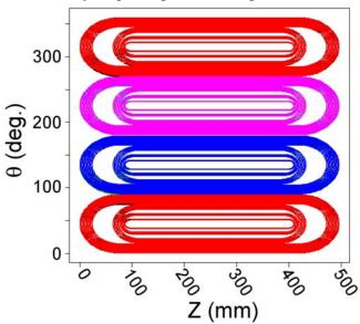
Figure 2.1: Sample Double Layer Quadrupole Coil Winding Pattern.
