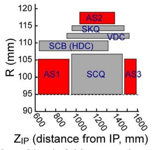
**Figure 3.1. Coil Layout Schematic.** Coil dimensions, conductor type and number of layers are given in Tables 3.1 and 3.2.
