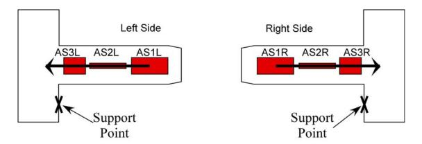
**Figure 5.1: Anti-Solenoid Longitudinal Force Diagram.** Net Longitudinal force on right and left sides is equal in magnitude and opposite in direction since current flows with the same handedness on right/left sides but the BES-III radial field reverses on right and left sides.
