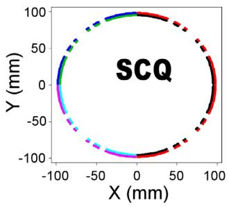
Figure 2.2: Sample Double Layer Quadrupole Coil Cross Section.
