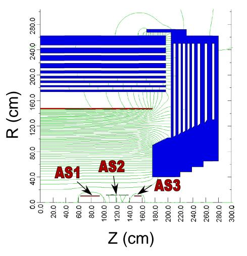
$I_{main} = 1120 \text{ A}$   $N_{AS1} = 732 \text{ turns}$   $N_{AS2} = 260 \text{ turns}$   $N_{AS3} = 280 \text{ turns}$   $N_{Tot} = 1272 \text{ turns}$   $I_{Tot} = 78 \text{ m H}$
