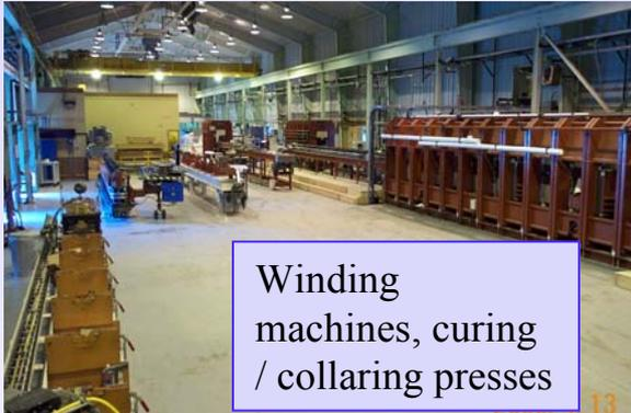
Winding machines, curing / collaring presses
