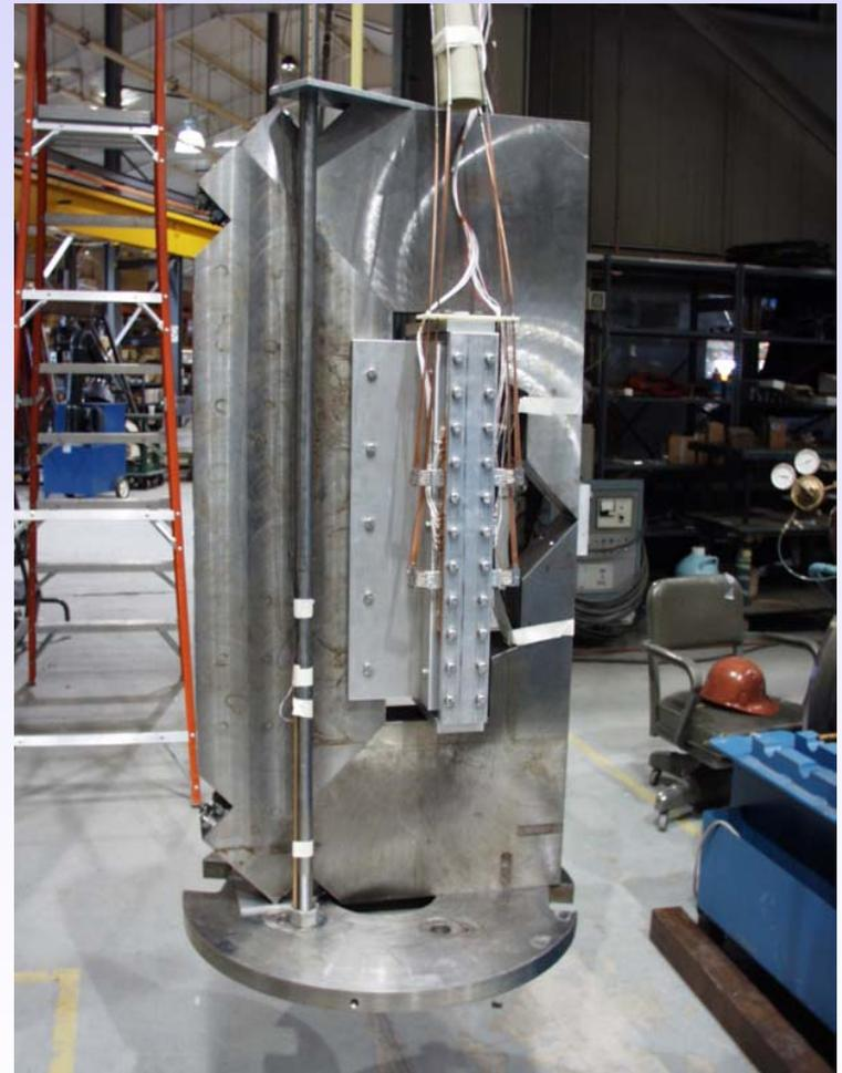
6 layer coil going for test in VTF
