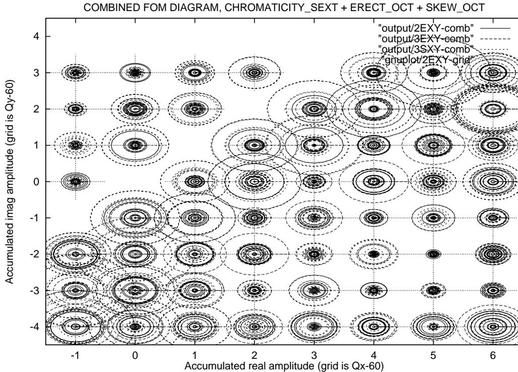
**Figure 7:** FOM values (plotted as ellipses centered on integer tune values  $(Q_x, Q_y)$ ), with chromaticity sextupoles plus erect octupole plus skew octupole systematic errors, all superimposed. Smallest blobs of ellipses are best. No points are plotted on the diagonal, which is hopelessly bad.
