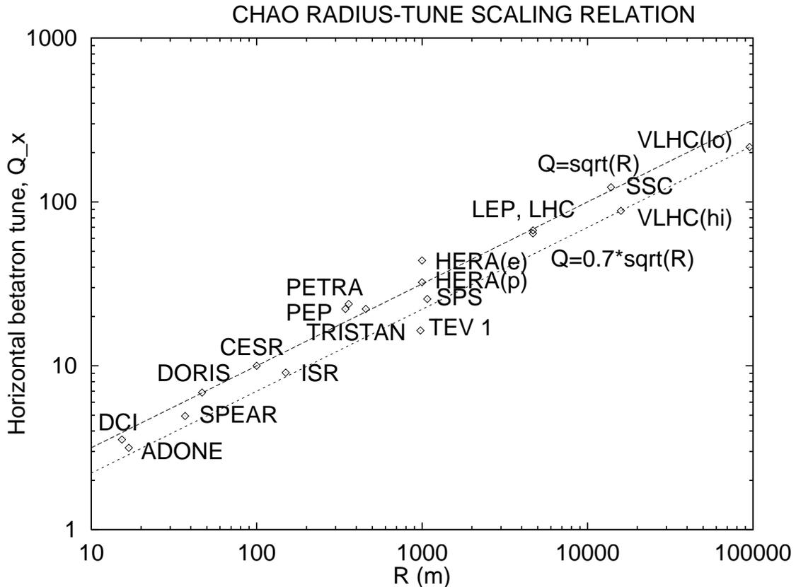
**Figure 2:** Empirical relation  $Q \sim R^{1/2}$  between radius  $R$  and tune  $Q$  for existing high energy accelerators. Copied from Chao. The lower line has been added because the focusing seems to be systematically lower for proton than for electron accelerators. High and low field VLHC design options have been placed on the curve extrapolated to large  $R$ .
