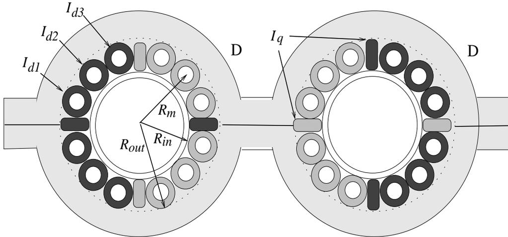
**Figure 3:** Suggested current distribution for ironless, “end-free”, combined function VLHC magnets. There are three independent bend-like currents,  $I_{d1}$ ,  $I_{d2}$ ,  $I_{d3}$ , and one quad-like current  $I_q$ .
