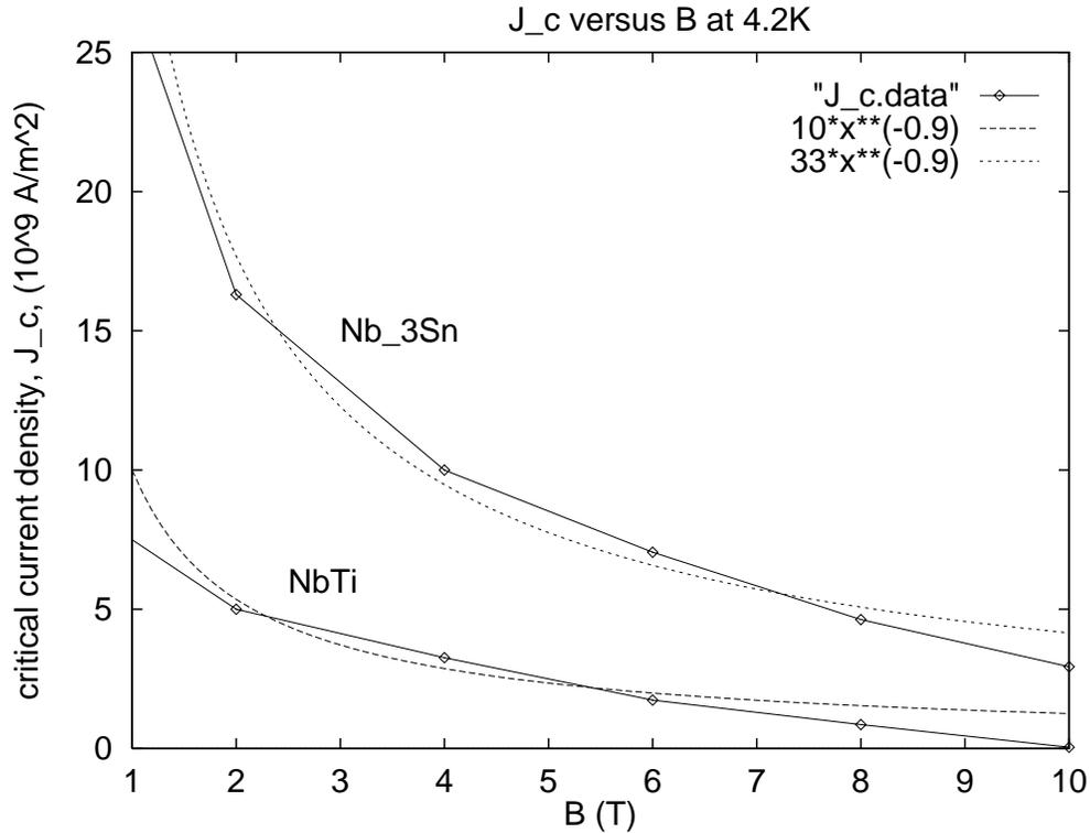
**Figure 4:** Critical current for NbTi and Nb<sub>3</sub>Sn at 4.2K, over likely range for  $B$ .
