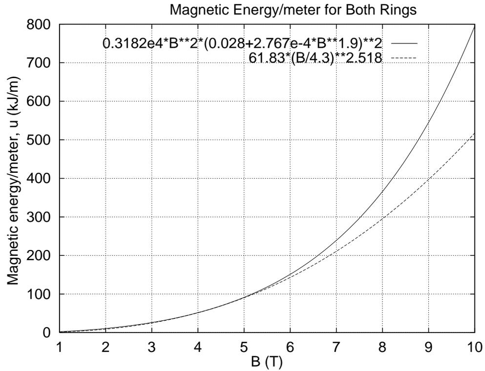
**Figure 5:** Stored energy per meter  $u$  (both rings). Also shown is a fit to the dependence  $u \sim B^m$ , yielding  $m = 2.518$ .
