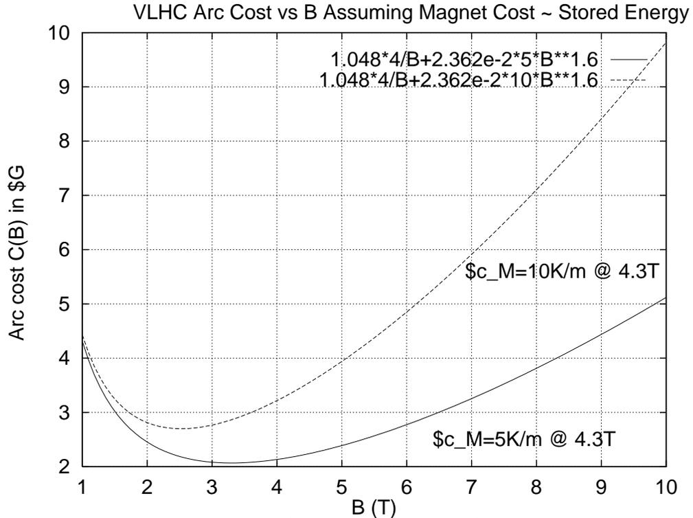
**Figure 6:** Arc cost  $C_T + C_M$  (tunnel and magnet) in billions of dollars assuming magnet cost is proportional to stored magnetic energy.
