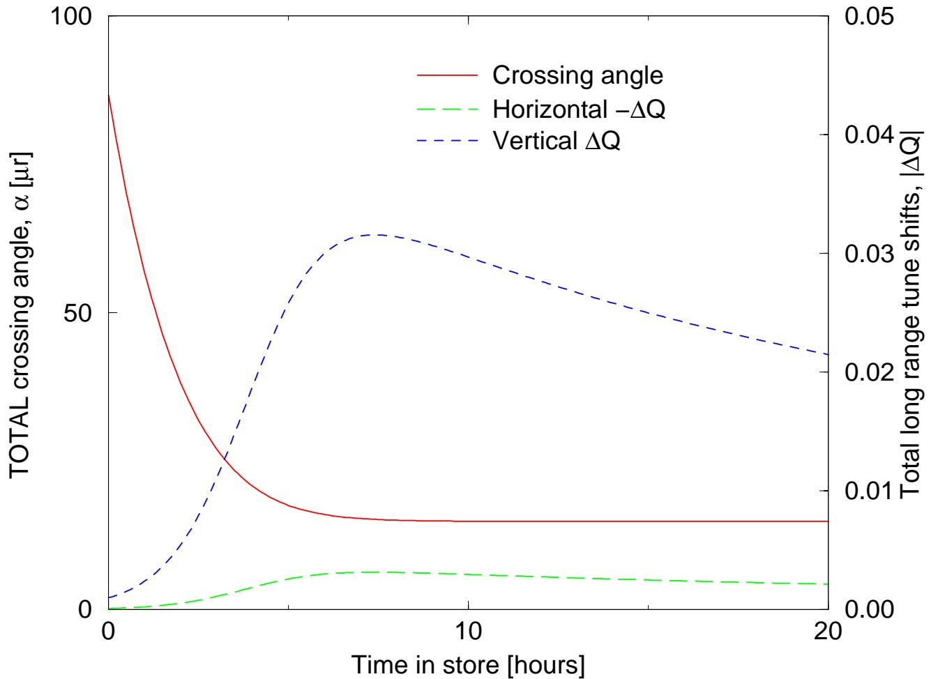
The VERTICAL long range tune shift  $\Delta Q_y$  is much larger than the horizontal:
