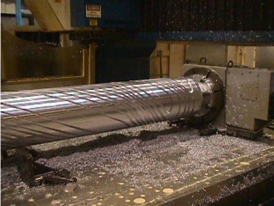
Figure 7. Machined inner coil support tube
