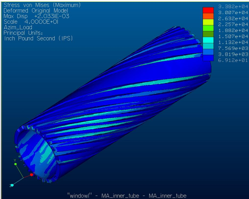
Figure 8. Inner Tube Stress
