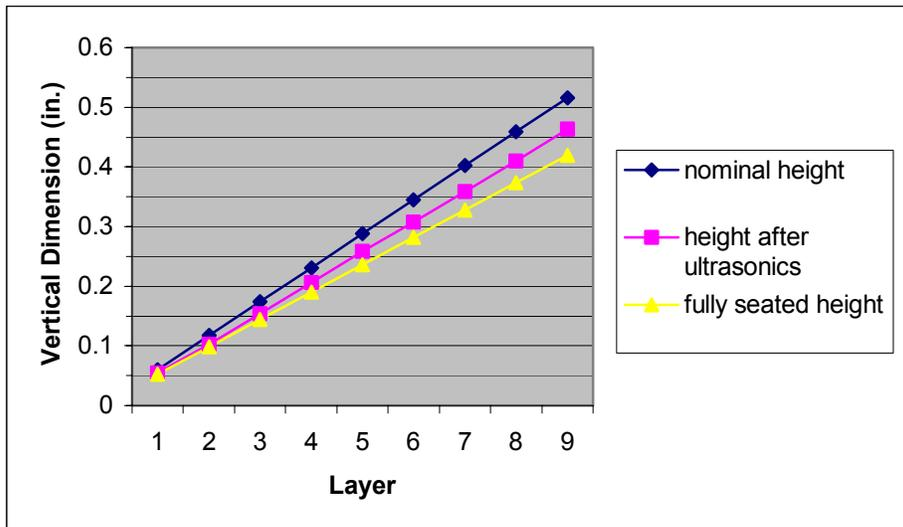
Figure 14. Comparison of Cable Seating Depths
