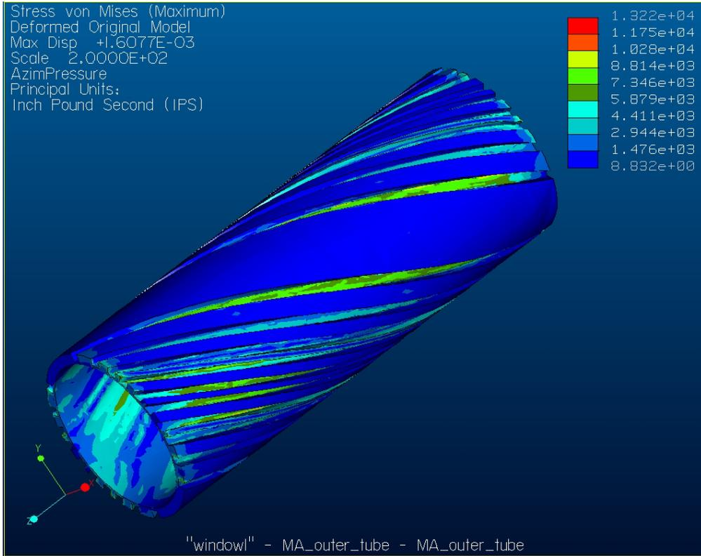
**Figure 10. Outer Tube Stress**
