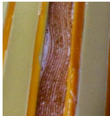
Figure 13. Cable positioning error
