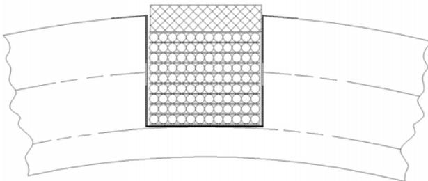
Figure 12. Coil Block cross-section
