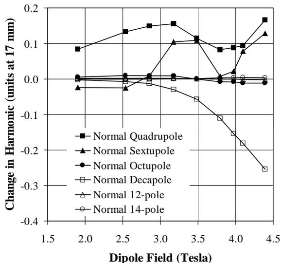
Figure 2: Saturation behaviour of various harmonics in D4A magnets, calculated using POISSON.
