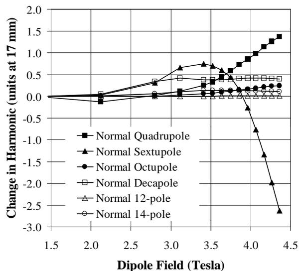
Figure 6: Calculated saturation behaviour of various harmonics in D3A magnets using an iron key.
