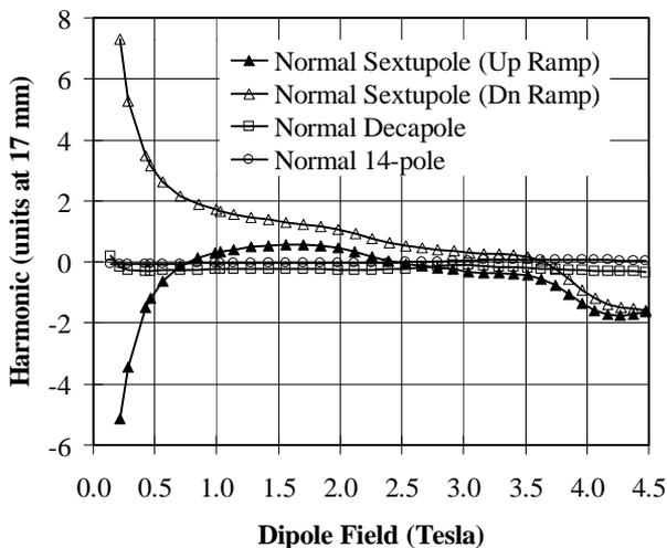
Figure 5: The measured current dependence of harmonics in a typical RHIC arc dipole, DRG107.
