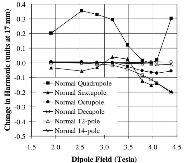
Figure 3: Saturation behaviour of various harmonics in D4B magnets, calculated using POISSON.
