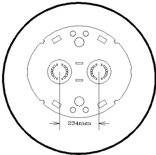
Figure 1: D4A cold mass inside the LHC cryostat.
