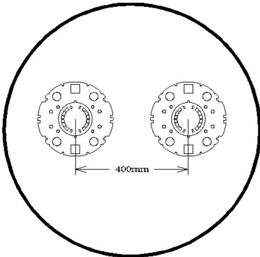
Figure 4: Two RHIC-type cold masses inside a LHC cryostat to give a D3A magnet. The D3B magnets are similar, except that the separation between the two beams is 382 mm.
