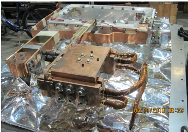
Figure 3: Underside of Magnet Lid
