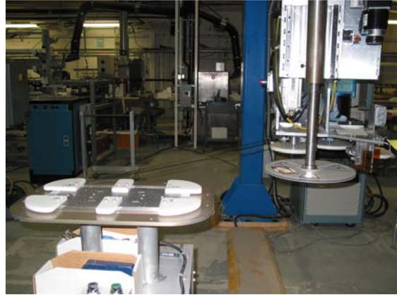
Fig. 4. A coil being wound with the newer computer controlled winding machine that is more efficient and provides better control, analysis and recording of winding parameters.
