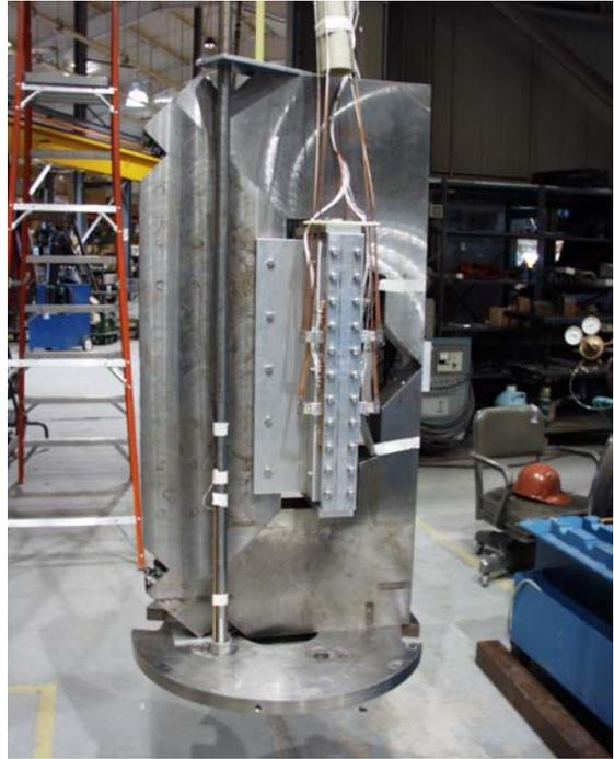
Fig. 8. Magnetic mirror model magnet, just before the test. The expected operating temperature in RIA will be in the range of 20 K to 40 K, depending on the magnet performance and overall optimization of the system that includes the cost of the large amount of energy removal from the magnet.
