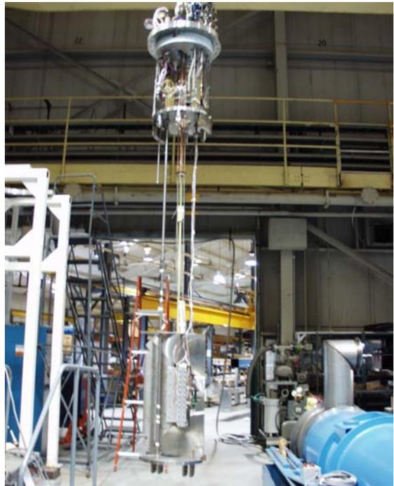
Fig. 9. Magnetic mirror model magnet with top hat (top) during its transport to the test station. At the test facility, the magnet can be tested in a wide range of temperature (4.2 K to 80 K).
