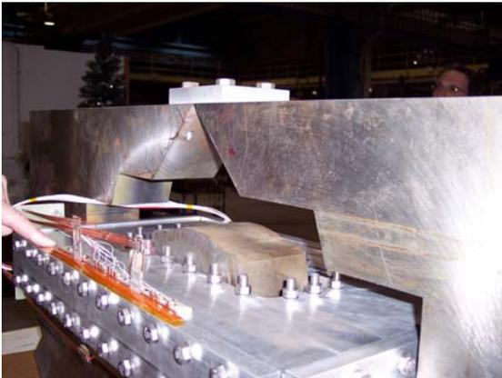
Fig. 7. Coils in their support structure and with the pole iron (in the middle, inside the structure), magnetic mirrors (two on the upper side with 45 degree angles on either side of the vertical axis) and iron return yoke.
