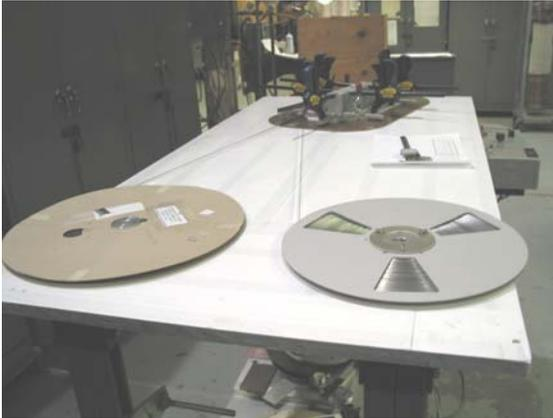
Fig. 3. A coil being made by co-winding HTS tape (on right) and stainless steel insulating tape (left). This is wound using a first generation winding machine that could be quickly set-up.
