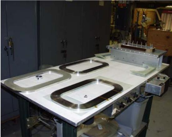
Fig. 5. Three pairs of coils (six coils) for the magnetic mirror model. These coils are made with HTS tape (nominal 4.2 mm wide and 0.3 mm thick) and insulating stainless steel tape (nominal 4.6 mm wide and 0.04 mm thick).
