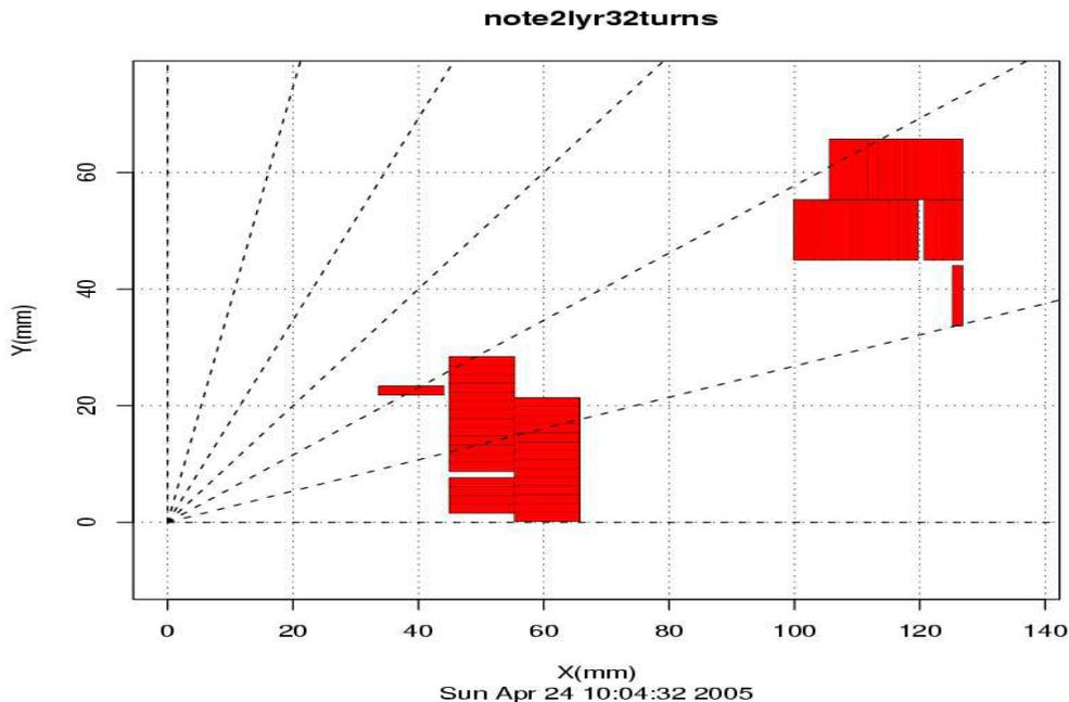
Fig. 4. An octant of 2 layer, 90 mm aperture LARP quadrupole design optimized for field quality using RACE2DOPT. The optimized harmonics are essentially zero.
