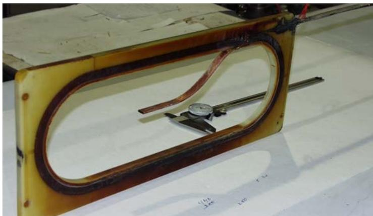
Fig. 2. An impregnated Nb<sub>3</sub>Sn coil with center space (island) free of any structure except for the splice. One would need similar coils for the modular design (the center space needs to be free of everything).
