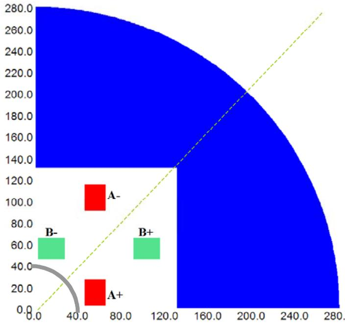
Fig. 1. A quadrant of the modular quadrupole design concept that also facilitates a modular R&D program. The design consists of two flat racetrack coil modules “A” and “B” that provide quadrupole symmetry in the cross-section (i.e. the two octants have mirror symmetry across the 45 degree line). The beam tube is shown in gray. The coils are interleaved in such a way that the integral harmonics in the ends will be small. All dimensions are given in mm.
