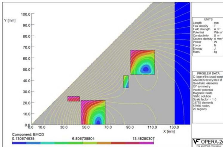
Fig. 3. An OPERA2d model of the octant of a 2 layer, 90 mm aperture LARP quadrupole design. The field lines are shown at the overall current density of 1000 A/mm<sup>2</sup>, which generates a gradient of ~284 T/m. The computed quench gradient is ~258 T/m for a critical current density of 3000 A/mm<sup>2</sup> (4.2K, 12T).
