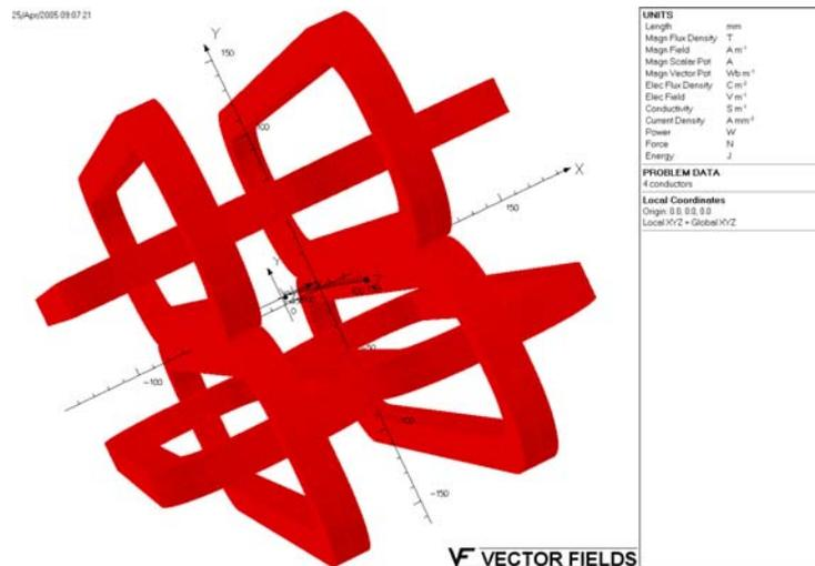
Fig. 5. Coils of modular design in a short magnet. The simplest way of interleaving coils creates a magnetic asymmetry in the ends between the horizontal and vertical planes and generates a non-zero octupole harmonic.
