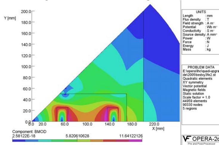
*Fig. 12. An alternate design with flat racetrack coils that utilizes many features and benefit of the modular design. However, the design is not efficient for high field magnets since it reduces the gradient and increases the peak field.*
