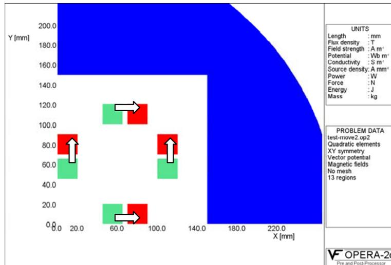
Fig. 10. In modular design the magnet aperture can be changed easily by changing the spacing between the coils. Coils in green location shows the case when the magnet aperture is 90 mm and the same coils in red location shows the case when the magnet aperture is 140 mm. Arrows indicates the direction in which two coils will have to move to increase aperture from 90 mm to 140 mm.
