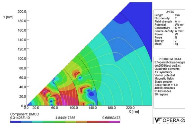
*Fig. 13. Another alternate design with flat racetrack coils that utilizes many features and benefit of the modular design. This design is also not efficient for high field magnets since this too reduces the gradient and increases the peak field.*
