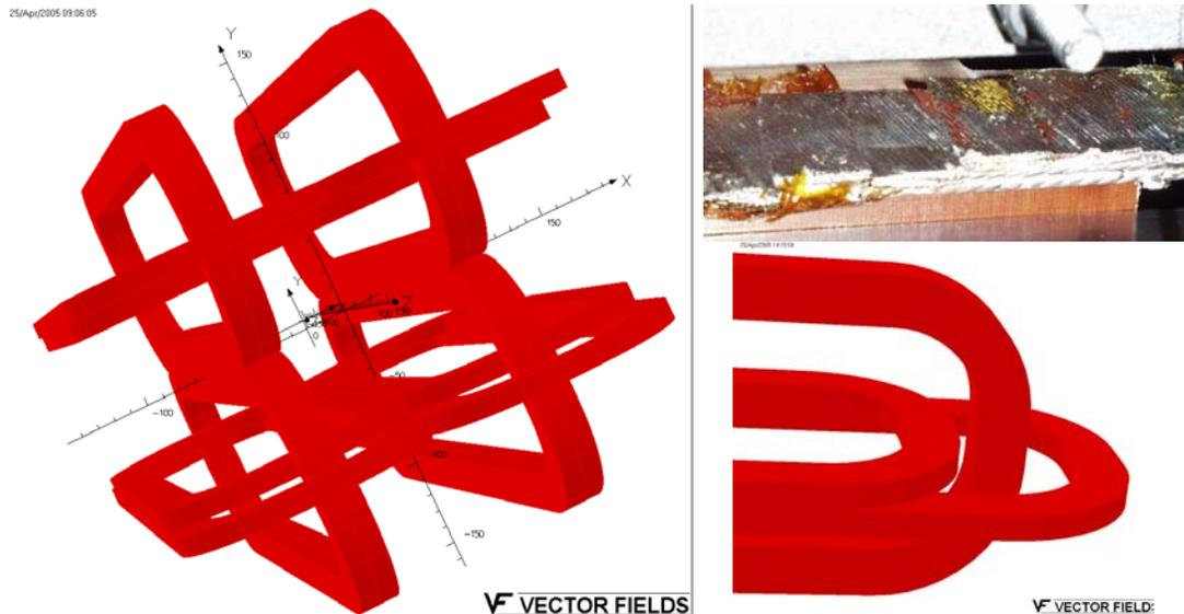
Fig. 7. Some interleaving coils are made smaller and some larger in an attempt to minimize magnetic asymmetry in the ends. Computer model on the left side shows the full magnet and on the lower-right shows the “lower-right” quadrant. The photo on the upper-right shows the type of perpendicular splice that may be used in splicing two single pancake coils of different lengths to a double pancake coil after all coils are put together.
