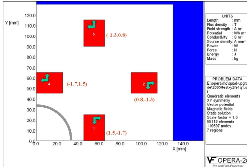
Fig. 9. Magnitude (Mega Newton/meter) and direction of Lorentz forces in blocks at  $\sim 235$  T/m gradient in the conceptual design of LARP 90 mm quadrupole.
