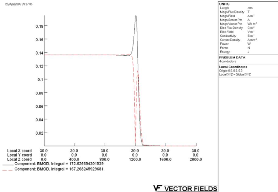
Fig. 6. The magnitude of the field as a function of axial position on the horizontal axis (black full line) and vertical axis mm (dashed red line) at a distance of 30 mm from the origin. The integral value is listed at the bottom of picture. The difference between the two integrals is the measure of integral asymmetry.
