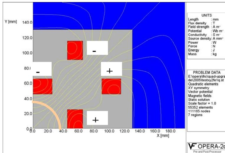
Fig. 11. Field lines in the first quadrant of modular design. Mirror iron can be placed on the X-axis and the Y-axis as the field lines are perpendicular there and an octant contains the complete coils.
