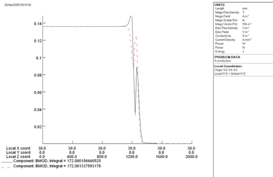
Fig. 8. The magnitude of the field as a function of axial position on the horizontal axis (black full line) and vertical axis mm (dashed red line) at a distance of 30 mm from the origin. The integral value is listed at the bottom of picture. The difference between the two integrals is the measure of integral asymmetry. One can see that the integral asymmetry is practically eliminated by adjusting the length of the coils. Integral harmonics will be optimized by 3-d coil optimization codes.
