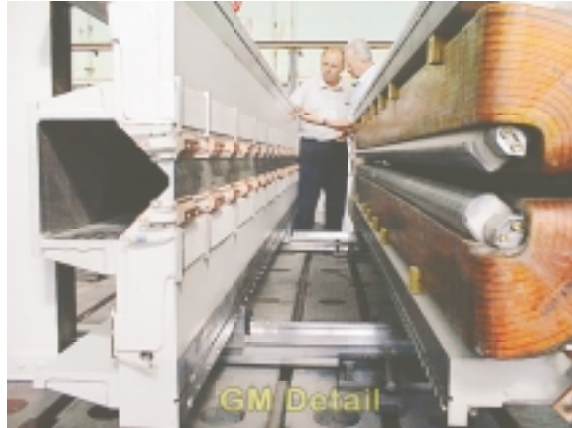
GM, the HERA Luminosity Upgrade Magnetic Septum Quadrupole (MSQ)
