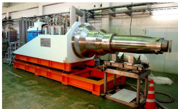
Figure 1: SuperKEKB left side cryostat at KEK.
