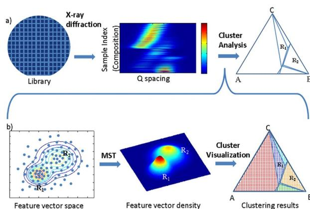
Figure 8: Machine learning strategies in high-throughput experiments searching for rare-earth-free permanent magnets.
