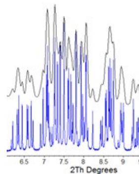
Figure 9: High resolution diffraction patterns of Gadolinium and Uranium based Salt Inclusion Materials (SIMs) for use as nuclear waste forms. Top: NSLS-II 28ID data. Bottom: high resolution APS 11-BM data. Courtesy of S. Gill (BNL) and G. Morrison (U. South Carolina).
