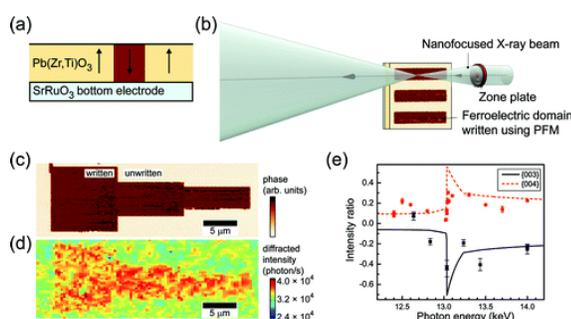
Figure 12: Reversed polarization domain in a  $\text{Pb}(\text{Zr,Ti})\text{O}_3$  ferroelectric thin film. (b) X-ray domain imaging based on a scanning 50 nm diameter probe beam. (c) piezoresponse force microscopy image and (d) map of diffracted X-ray intensity using  $\{002\}$  reflections of a domain pattern.
