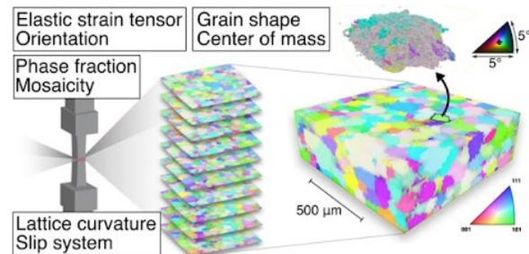
Figure 5: Near-field 3D X-ray Diffraction Microscopy (1  $\mu\text{m}$  resolution, 1 mm<sup>3</sup> FOV). Courtesy of A. Bucsek.
