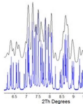
Figure 9: High resolution diffraction patterns of Gadolinium and Uranium based Salt Inclusion Materials (SIMs) for use as nuclear waste forms. Top: NSLS-II 28ID data. Bottom: high resolution APS 11-BM data. Courtesy of S. Gill (BNL) and G. Morrison (U. South Carolina).
