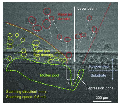
Figure 4: X-ray image of powder spattering during laser single track scanning.<sup>1</sup>
