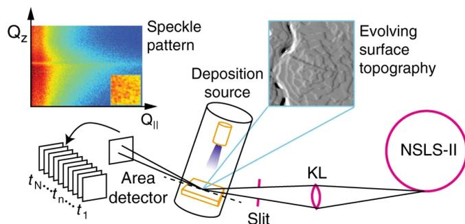
Figure 7: Coherent scattering characterization of  $C_{60}$  thin-film deposition. (111)-oriented crystalline mounds form via nucleation events captured by the intensity distribution of scattered x-rays.
