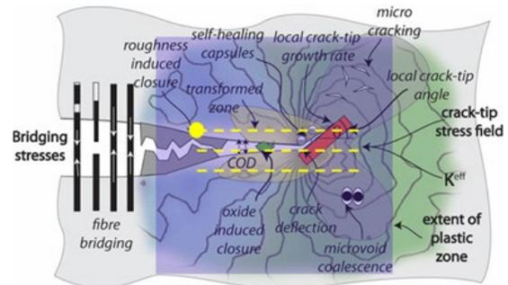
Figure 11: Simultaneous micro-diffraction (yellow) and full-field imaging (blue) for crack growths dynamics.
