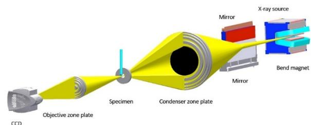
**Figure 17.** CAD showing XM-2 source, mirrors, optics and the beam path from the bend magnet source, through the specimen, and onto the detector.
