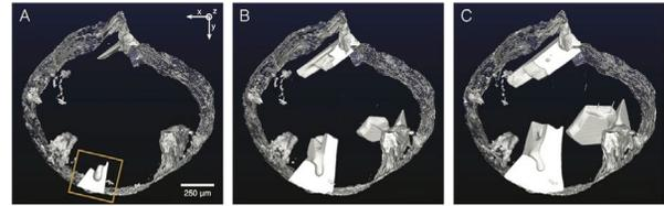
Figure 10: 3-D reconstructions of Si particle growth. White regions are the primary Si particles, translucent light gray region is the oxide skin and the dark blue background is the Cu-enriched liquid. Three images represent (A) 2079 s (875 °C), (B) 4261 s (839 °C) and (C) 8031 s (776 °C).
