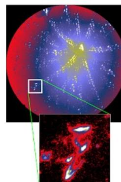
Figure 13. 3D X-ray micro-diffraction using either the triangulation or the differential aperture X-ray microscopy techniques.<sup>1</sup>
