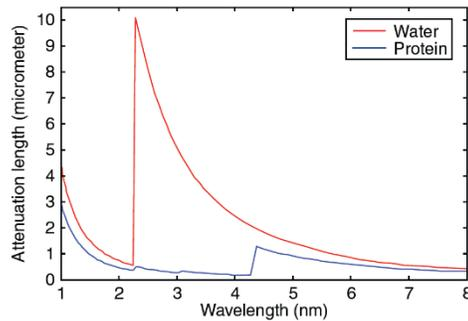
**Figure 18.** Attenuation of ‘water window’ soft x-rays by protein and water.
