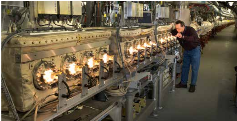
Electronic “pickups” of RHIC’s stochastic cooling system
