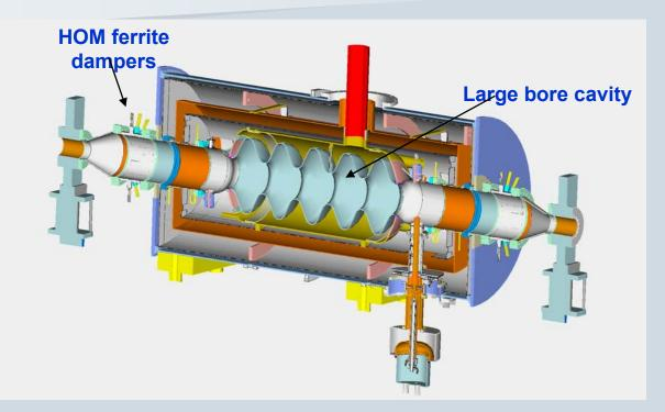
703.75 MHz 5-cell cavity designed in BNL for e-cooling and eRHIC
