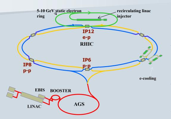
The e-ring design development led by MIT-Bates. Technology similar to used at B-factories.
