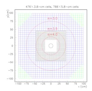
**Figure 6:** Front view of the STAR Forward Meson Spectrometer (FMS). The FMS consists of 1264 Pb-glass cells and cover the pseudorapidity region  $2.5 < \eta < 4$ . The FMS greatly expands STAR's acceptance for mesons decaying into photons and for meson coincidences in a kinematic region where particle production is dominated by contributions that are sensitive to low-*x* gluons in the Au nucleus.
