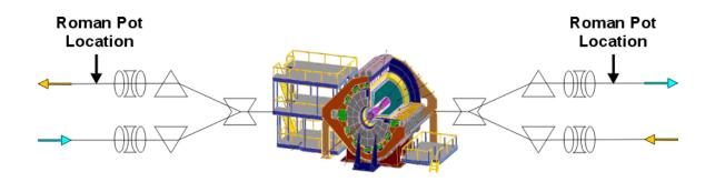
**Fig. 19**. The Roman pots of the pp2pp experiment in the STAR interaction region, with the arrows indicating proposed location. At each location one Roman Pot station is horizontal and one vertical.
