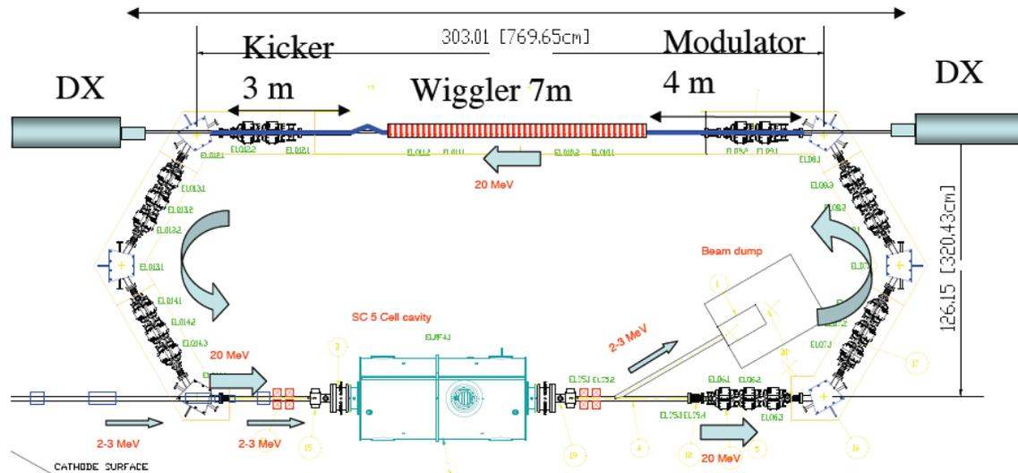
**Planning proof of principle demo of coherent e-cooling in RHIC, using ~20 MeV e from ERL already being developed + 40 GeV/N Au beams.**
