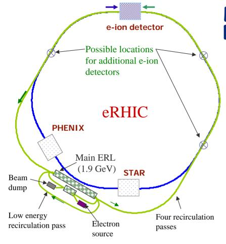
Subsequent stages/ alternative layouts could increase e-beam & ionbeam energies and L from nominal 10 × 250 GeV, ~3 × 10<sup>33</sup> cm<sup>-2</sup>s<sup>-1</sup> e+p
