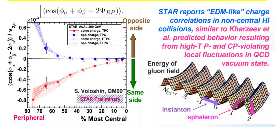
Statistically significant signal must average over many events and local "bubbles" with possibly opposite signs of CPV and chiral imbalance  $\Rightarrow$  signal is P- and CP-even, subject to contamination by mundane effects.
