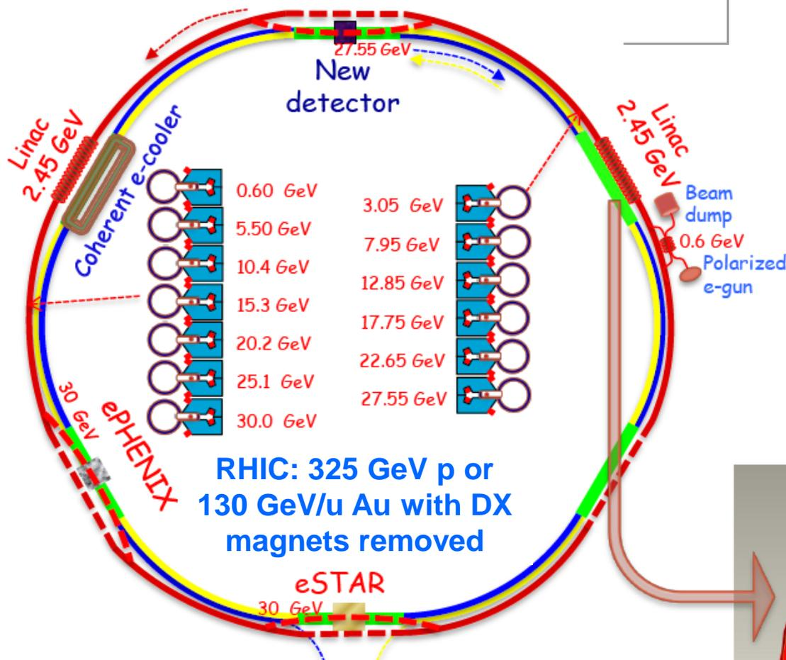
✓ All-in tunnel staging approach uses two energy recovery linacs and 6 recirculation passes to accelerate the electron beam.
