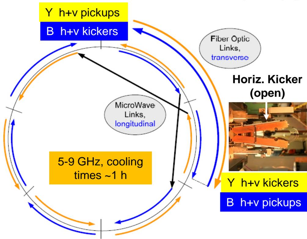
➤ **RHIC breakthrough in bunched-beam stochastic cooling overcomes intrabeam scattering limits, facilitates ~x10 improvement in heavy-ion collision rates, 4 years earlier and at ~1/7 the cost envisioned in 2007 NP Long Range Plan.**
