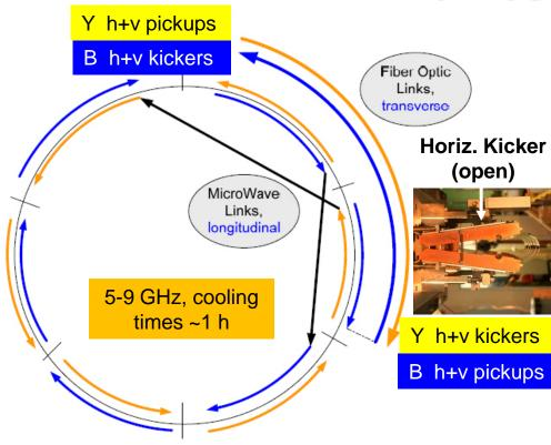
RHIC breakthrough in bunchedbeam stochastic cooling overcomes intrabeam scattering limits, facilitates ~x10 improvement in heavy-ion collision rates, 4 years earlier and at ~1/7 the cost envisioned in 2007 NP Long Range Plan.
