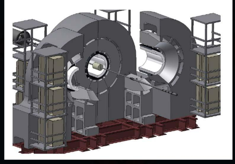
Major change to the PHENIX detector. Removal of outer PHENIX central arms, keep VTX inner tracking.
