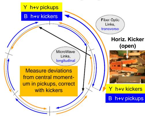
RHIC breakthrough in bunchedbeam stochastic cooling facilitates ~x10 improvement in heavy-ion collision rates, 4 years earlier and at ~1/7 the cost envisioned in 2007 NP Long Range Plan, saving ~\$80M
