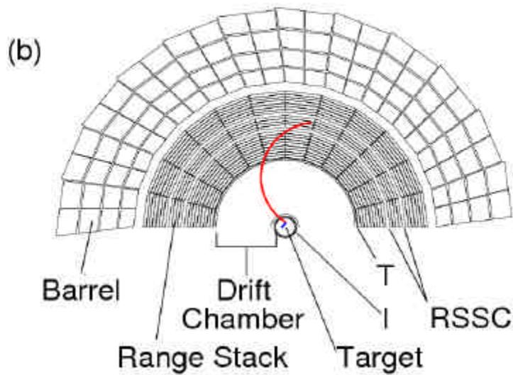
Figure 7 (a) Side and (b) end view of upper half of E949 detector
