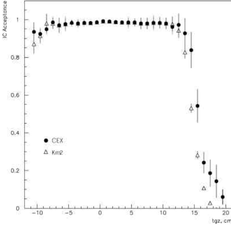
Figure 10 Acceptance of E787 target and trigger counters for charge exchange and  $K^+ \rightarrow \mu^+ \nu$  events.
