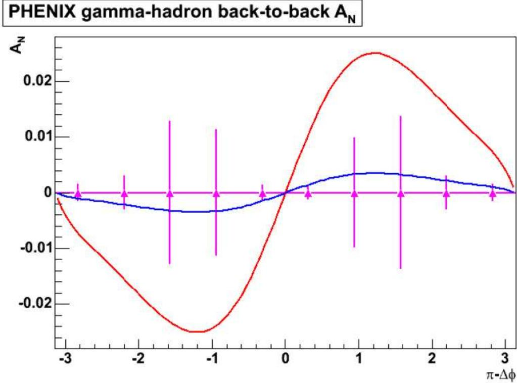
Figure 17: Expected sensitivity of  $A_N$  of back-to-back  $\pi^0$ -hadron pairs in the central arm. The theory lines are the maximal (red) and minimal (blue)  $A_N$  cited in Ref. [22], corresponding to estimates where the magnitude of the gluon Sivers function is equal to a parametrization of the d-quark Sivers distribution from E704  $A_N$  or to a case where the gluon Sivers function is identically zero, respectively.
