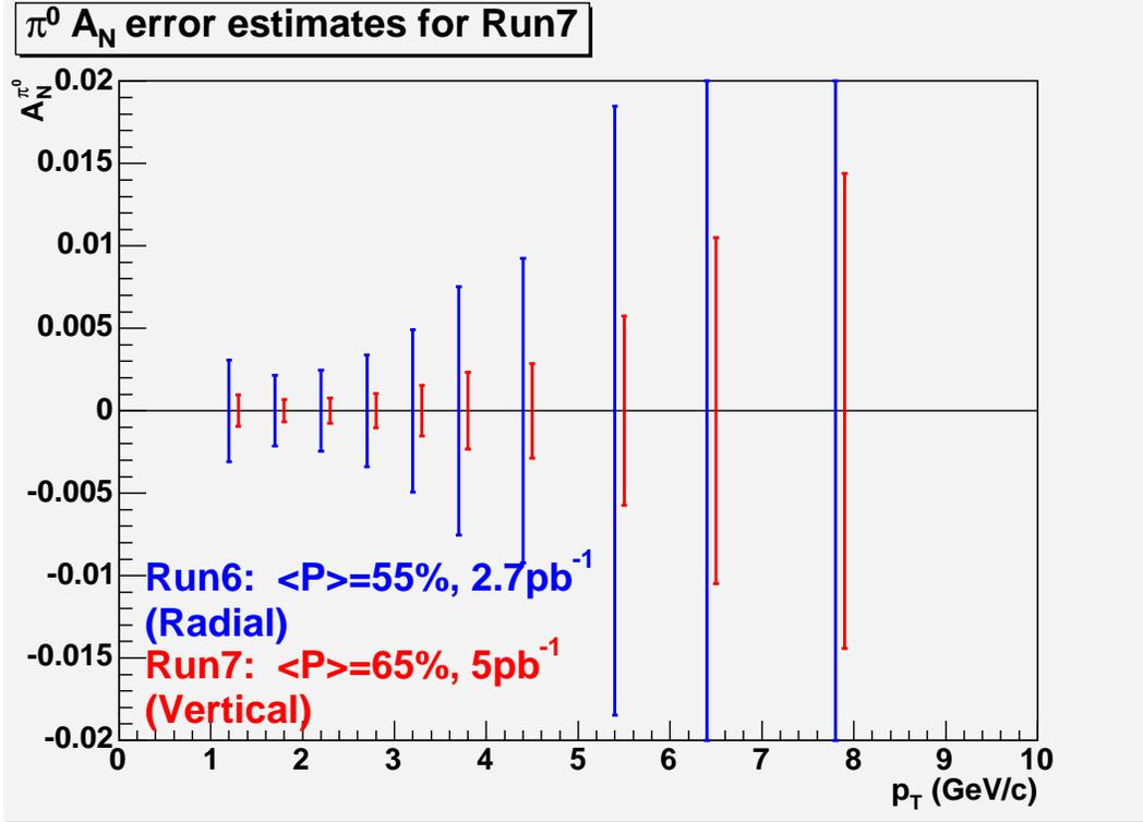
Figure 16: Projected  $A_N^{\pi^0}$  measurement in Run-6 and 7 in the central rapidity assuming our known analysis cut losses and beam polarization direction. Run-6 was estimated for radial transverse operation, while the Run-7 are shown assuming vertical transverse collisions at PHENIX.
