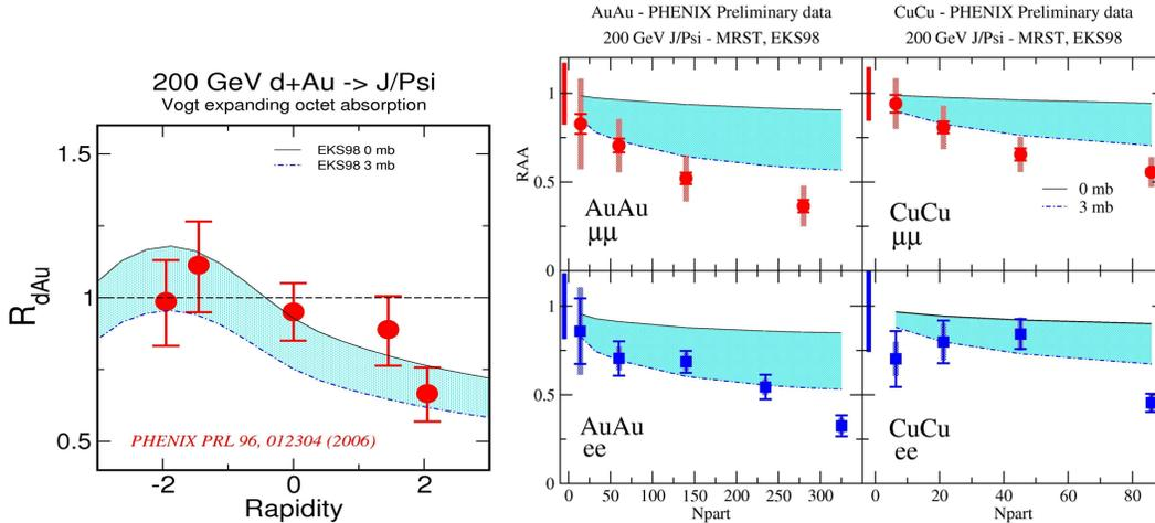
Figure 22: PHENIX Run-3 results[27] from  $\sqrt{s_{NN}} = 200$  GeV d+Au collisions for (left) the nuclear suppression factor  $R_{dAu}$  as a function of rapidity, compared to models incorporating various values of the absorption cross section and (right) the range of suppression factors allowed by the uncertainty in the absorption cross section, as compared to PHENIX Preliminary data from Au+Au and Cu+Cu collisions.
