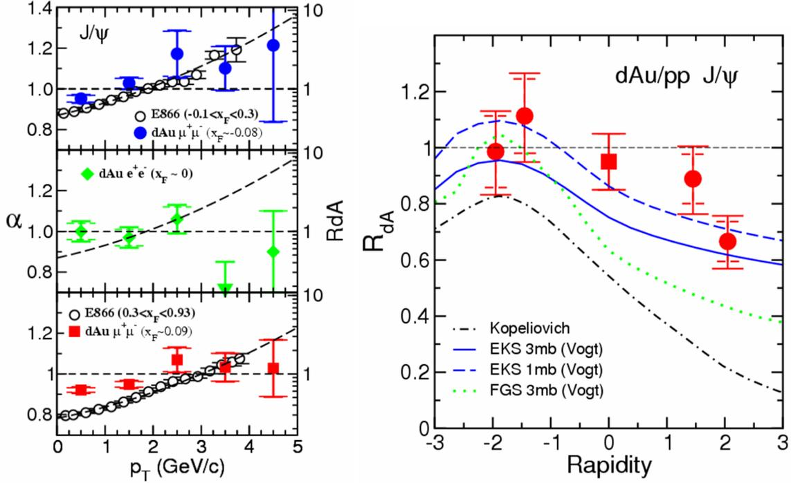
Figure 21: PHENIX Run-3 results[27] from  $\sqrt{s_{NN}} = 200$  GeV d+Au collisions for (left)  $J/\psi$  yields parameterized as  $A^\alpha$  as a function of transverse momentum compared to results from E866/NuSea[28] and (right) the nuclear suppression factor  $R_{dAu}$  as a function of rapidity, compared to various models of initial-state shadowing and final-state absorption[29, 30, 31].
