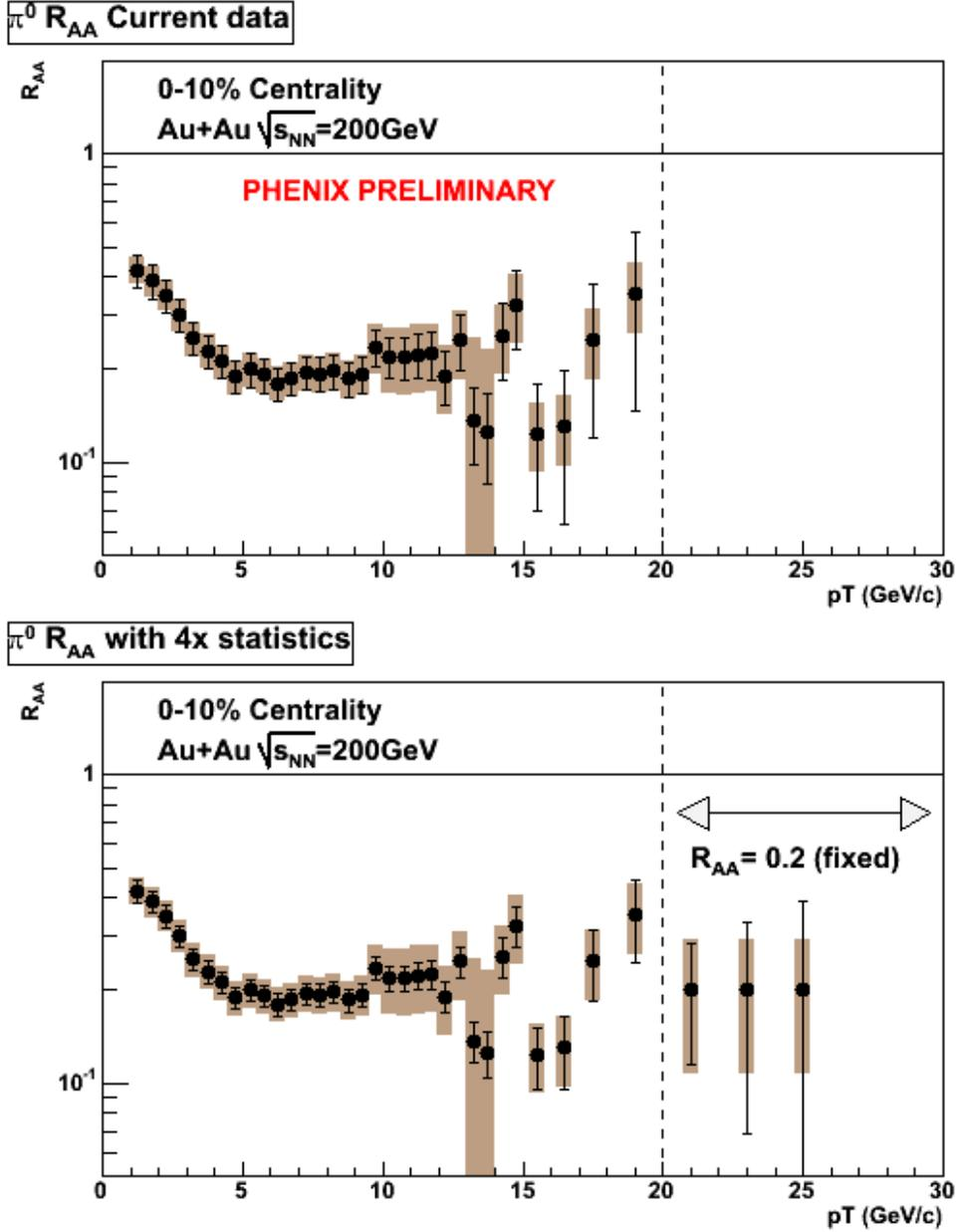
Figure 14: The PHENIX Preliminary nuclear suppression factor  $R_{AA}^{\pi^0}(p_T)$  from Run-4 (top plot) is compared to the improved precision and  $p_T$  reach made possible by the requested Run-7 Au+Au run (bottom plot).
