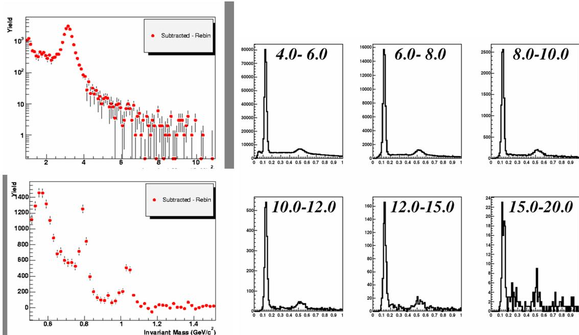
Figure 4: Results from Level-2 filtered data produced in quasi-real time by PHENIX during Run-6. Left Top: Invariant mass spectrum of  $\mu^+\mu^-$  pairs in the South Muon Arm. Left Bottom: Invariant mass spectrum of  $e^+e^-$  pairs in the Central Arms. Right: Invariant mass spectra of  $\gamma\gamma$  pairs for various  $p_T$  bins (in-plot label, in  $\text{GeV}/c$ ) in the Central Arms.
