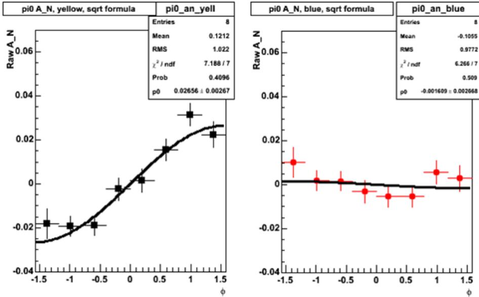
Figure 3: The raw  $\Phi$  asymmetry observed in the South Muon Piston Calorimeter for transversely polarized collisions in the Yellow beam (left) and the Blue beam (right). Pions incident upon the South MPC corresponds to large positive (negative)  $x_F$  for polarization in the Yellow (Blue) beam.
