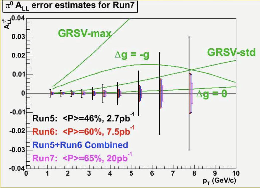
Figure 18: Projected  $A_{LL}^{\pi^0}$  measurement in Run-7. For comparison, estimations for previous measurements, including the recently finished Run-6 and the analyzed data set from Run-5 have been shown. The reduction of about 15% statistical sample due to analysis cuts has been applied to the Run-7 data set based on our knowledge of these from Run-5. Various scenarios of  $\Delta G$  based on GRSV fits[25] and their assumptions[26] are shown in green.
