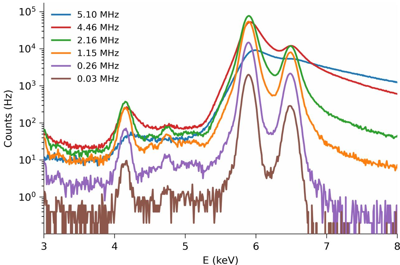
Analyzable spectra to about 2 MHz per channel.
