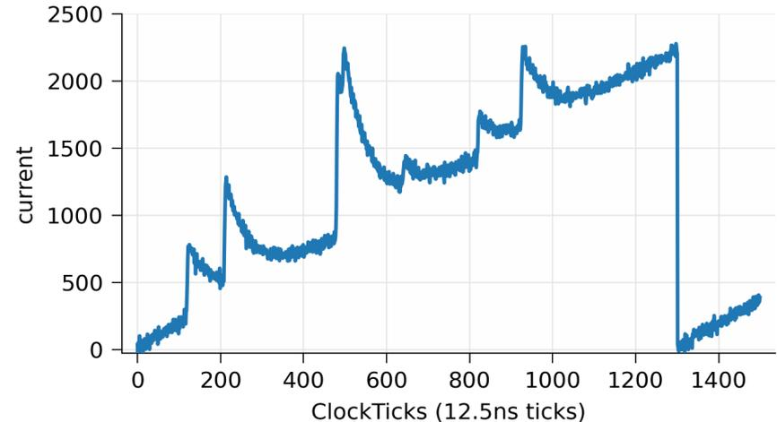
The detection and processing for each event takes some minimum time – an ***EventWidth*** so that the recommend way of estimating LiveTime is
