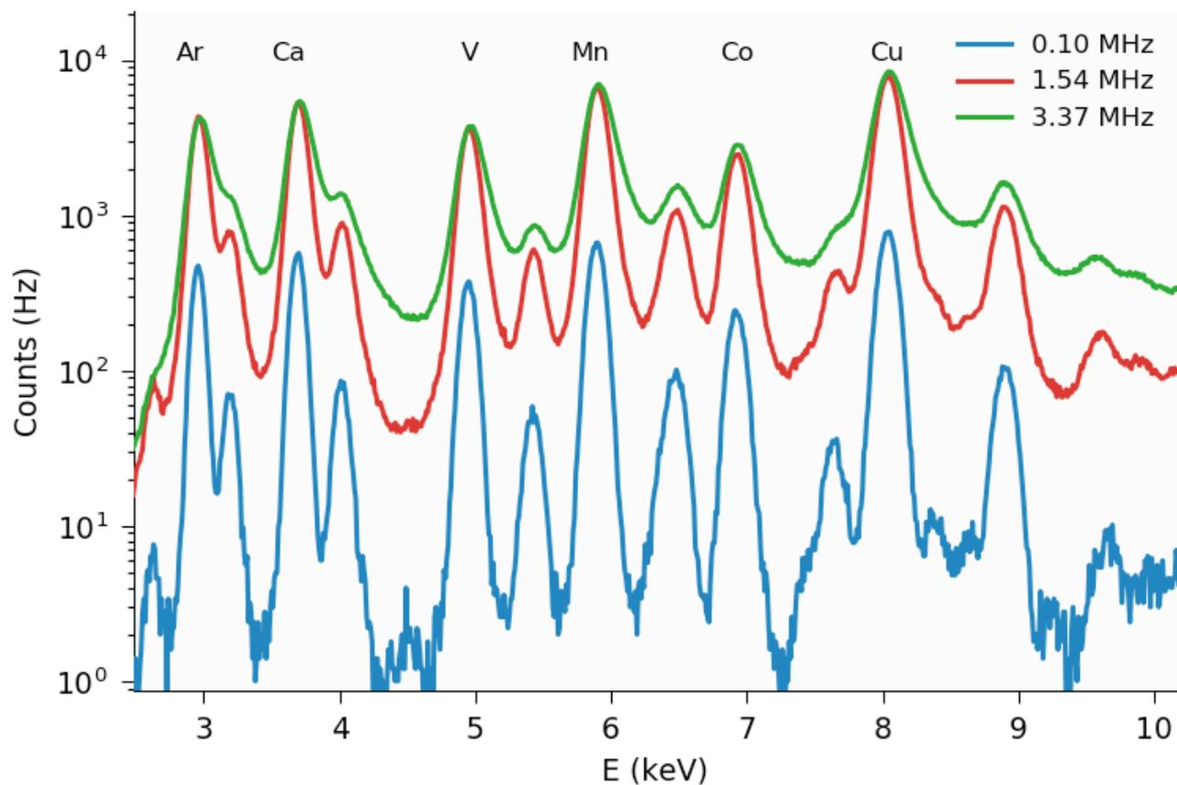
Analyzable spectra above 1.5 MHz per channel.
