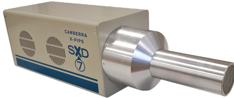
The detector runs at  $-80^{\circ}\text{C}$ , using Canberra's Cryo-Pulse pump and controller.
