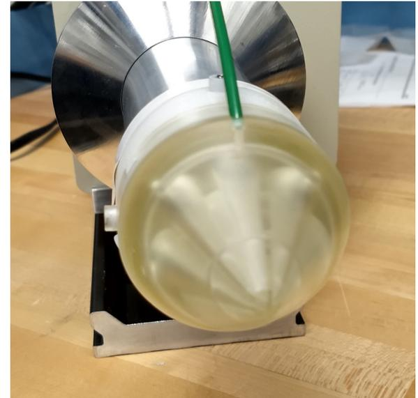
From a Similar collimator for ME-4, this will reduce background signals and window damage.
